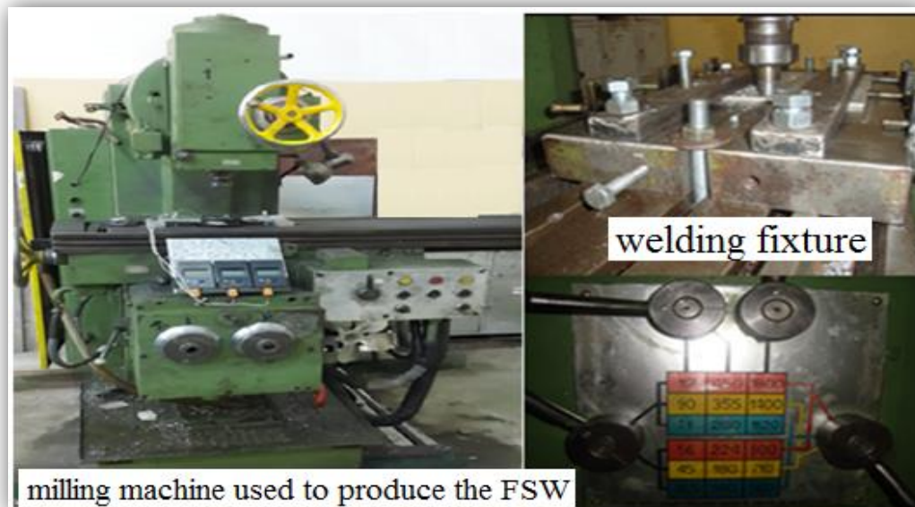
Figure (3): Universal of milling-machine (fixture and plate to be welded).
