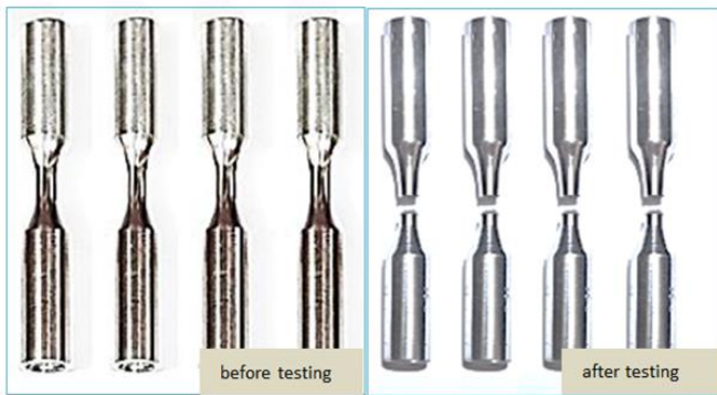
Figure 3. Samples of fatigue test specimens, both before and after testing.
