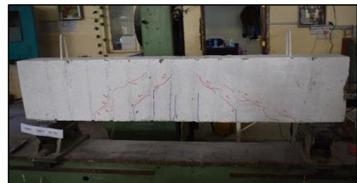
**Figure 18.** Crack patterns for B5-RS-T200
