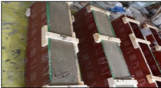
**Figure 3.** Beam specimens cast
