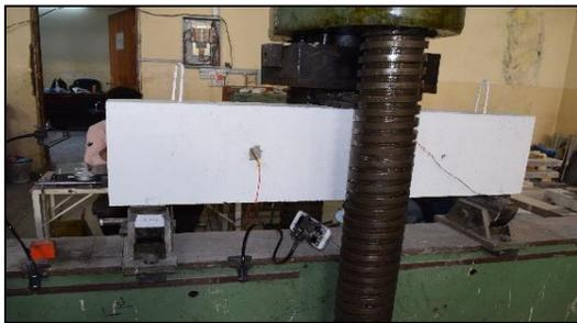
**Figure 5.** Beam specimens setup
