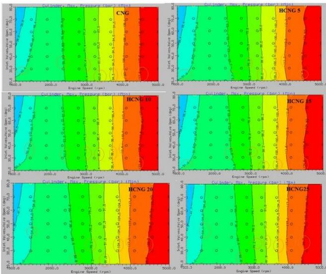
**Figure 9:** Cylinder gas pressure contours vs. different speeds at different blending ratios of hydrogen
