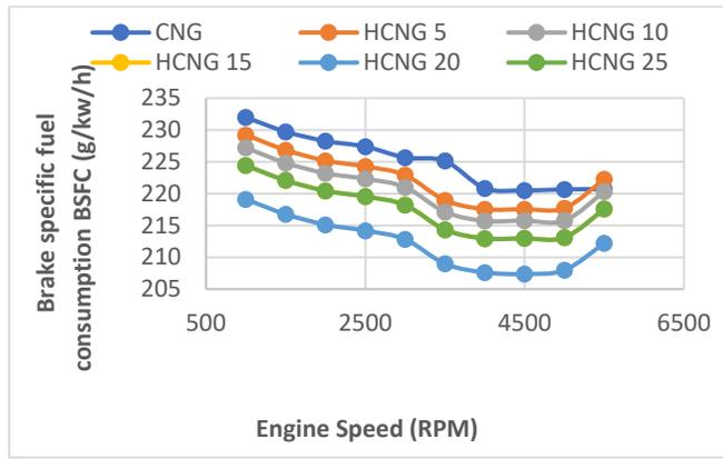
**Figure 4:** Variation in BSFC versus engine speed at different blending ratios of hydrogen
