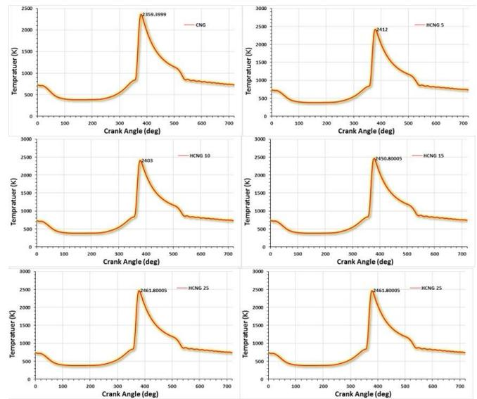
**Figure 6:** Temperature vs crank angle for different blending ratios of hydrogen at 1000 rpm
