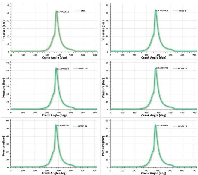
**Figure 5:** Pressure vs crank angle for different blending ratios of hydrogen at 1000 rpm
