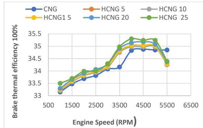
**Figure 2:** Variation in Brake thermal efficiency versus engine speed at different blending ratios of hydrogen
