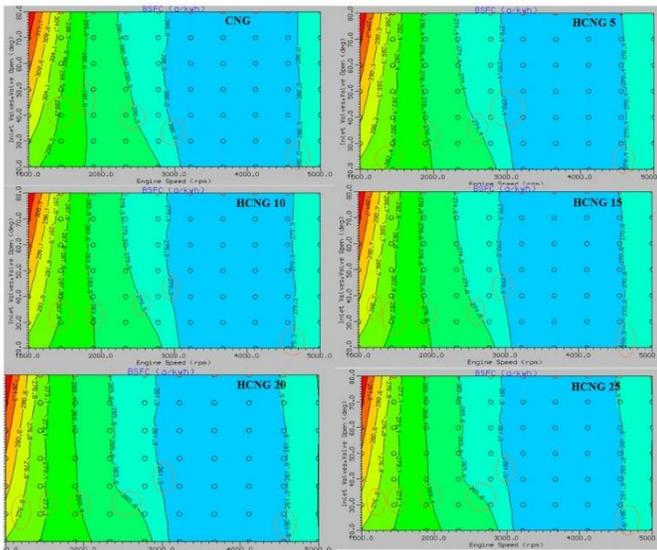
**Figure 8:** BSFC contours vs. different speeds at different blending ratios of hydrogen
