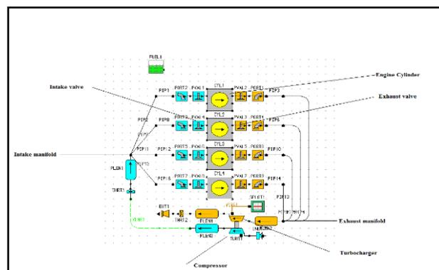
**Figure 1:** Engine model by LOTUS engineering software
