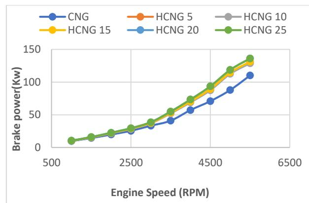
**Figure 3:** Variation in Brake power versus engine speed at different blending ratios of hydrogen
