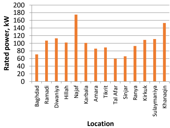
Figure 12. Rated power in the locations of Group (B) at 80 m using H-HAWT turbine.
