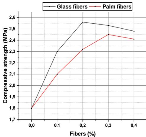
Figure 4. Compressive strength of samples.
