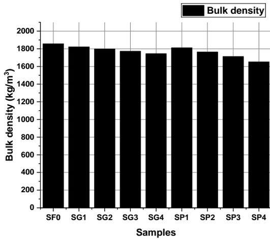
Figure 3. The change in bulk density when adding fibers.
