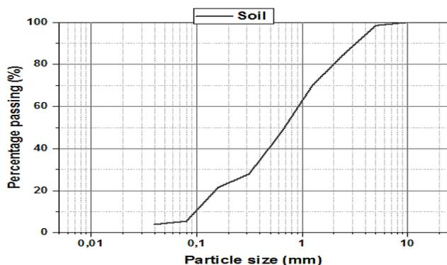
**Figure 1.** Soil particle analysis.
