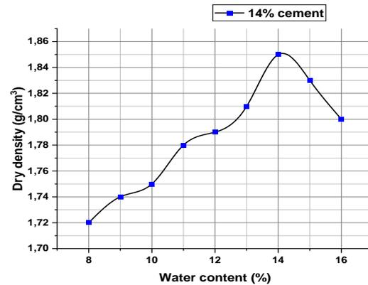
**Figure 2.** Optimum water content at 14% of cement.
