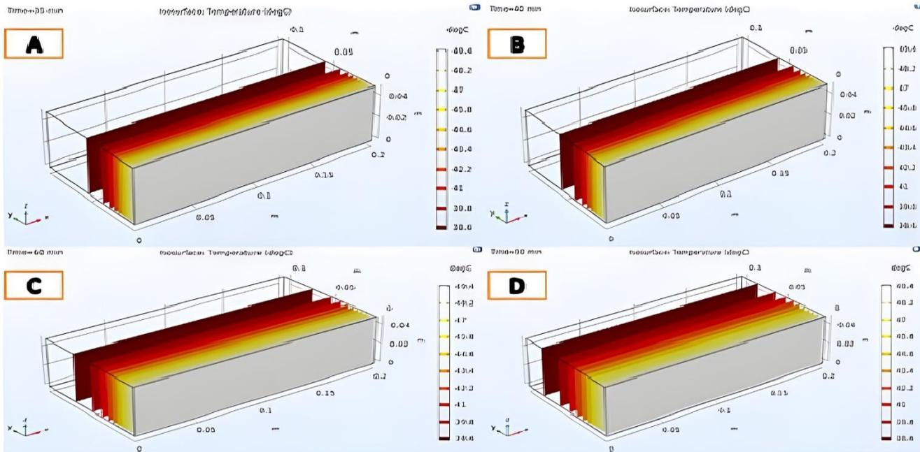
Figure 7. Heat transfer in the sample SF0.
