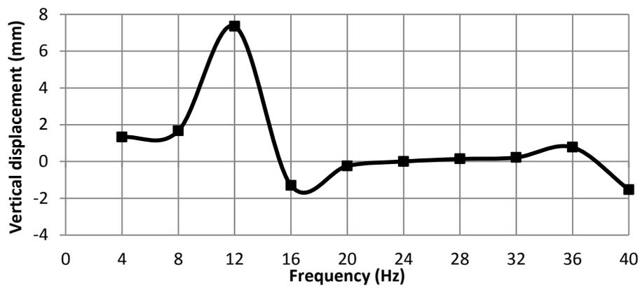
Figure 18. Vertical displacement (at the point of maximum displacement under static loading) embedded in soil due to low harmonic loading range.
