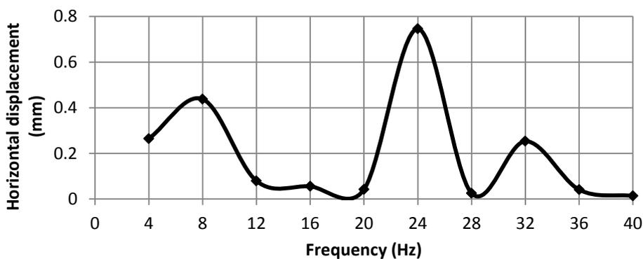
Figure 8. Horizontal displacement of the pile head (node 788) due to low harmonic loading range.
