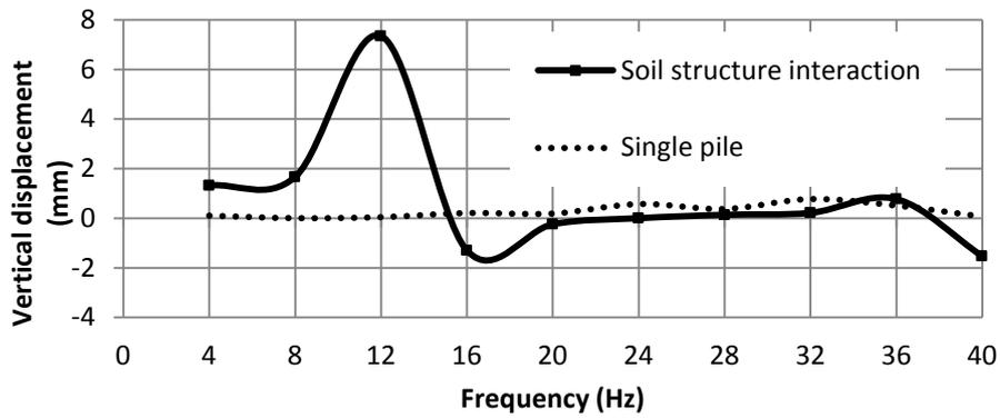
Figure 24. Vertical displacement (at the point of maximum displacement under static loading) embedded in soil compared with single pile due to low harmonic loading range.
