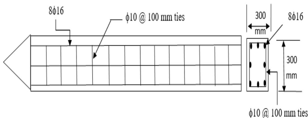
Figure 1. Pre-cast driven pile.
