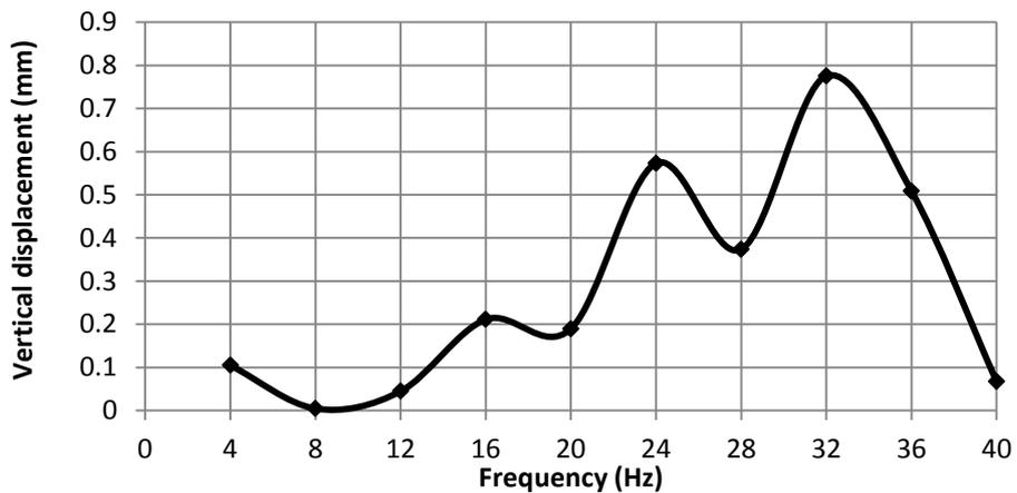
Figure 7. Vertical displacement (at the point of maximum displacement under static loading) due to low harmonic loading range.
