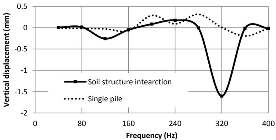
Figure 26. Vertical displacement (at the point of maximum displacement under static loading) embedded in soil compared with single pile due to medium harmonic loading range.
