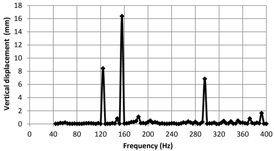
Figure 10. Vertical displacement (at the point of maximum displacement under static loading) due to medium harmonic loading range.
