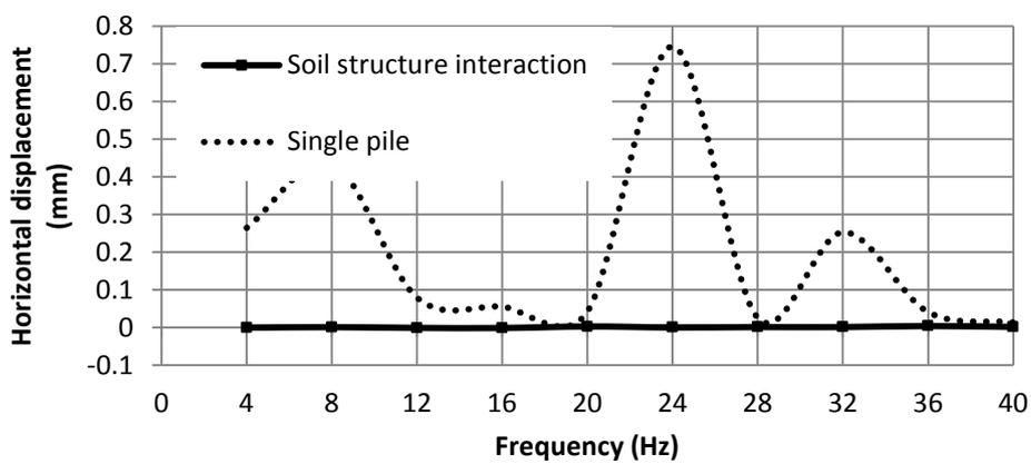
Figure 25. Horizontal displacement of the pile head (node 788) embedded in soil compared with single pile due to low harmonic loading range.
