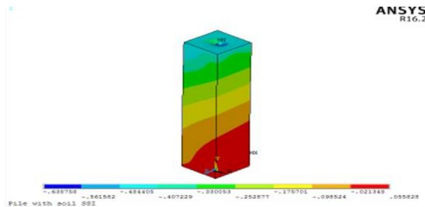
Figure 17. Lateral displacement along pile embedded in soil due to maximum static loading.
