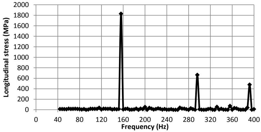
Figure 12. Longitudinal stress of the pile head (node 788) due to medium harmonic loading range.
