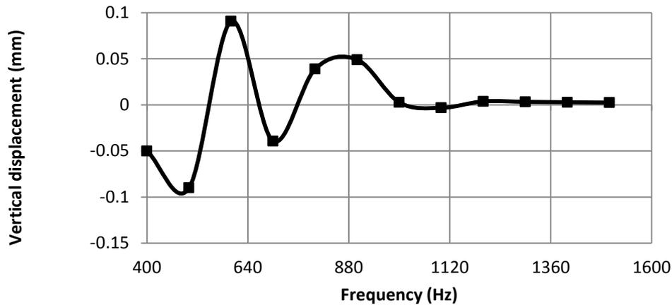
Figure 22. Vertical displacement (at the point of maximum displacement under static loading) embedded in soil due to high harmonic loading range.
