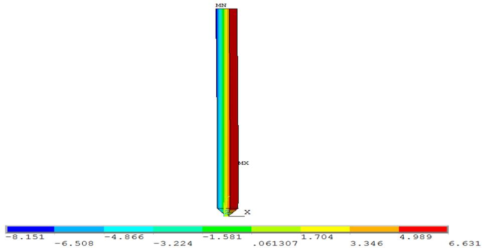
Figure 6. Horizontal displacement of pile due to static loading "u<sub>x</sub>".
