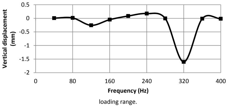
Figure 20. Vertical displacement (at the point of maximum displacement under static loading) embedded in soil due to medium harmonic loading range.
