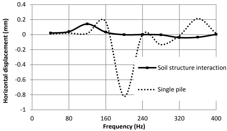
Figure 27. Horizontal displacement of the pile head (node 788) embedded in soil compared with single pile due to medium harmonic loading range.
