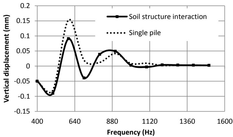
Figure 28. Vertical displacement (at the point of maximum displacement under static loading) embedded in soil compared with single pile due to high harmonic loading range.
