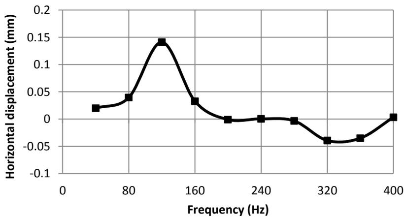
Figure 21. Horizontal displacement of the pile head (node 788) embedded in soil due to medium harmonic loading range.
