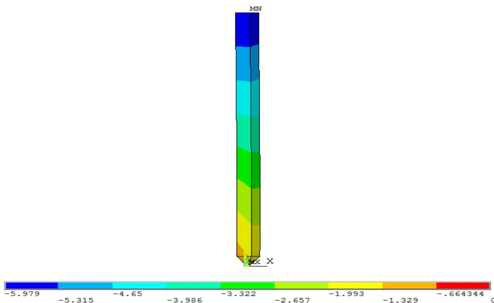
Figure 5. Vertical displacement along pile due to static loading "u<sub>y</sub>".
