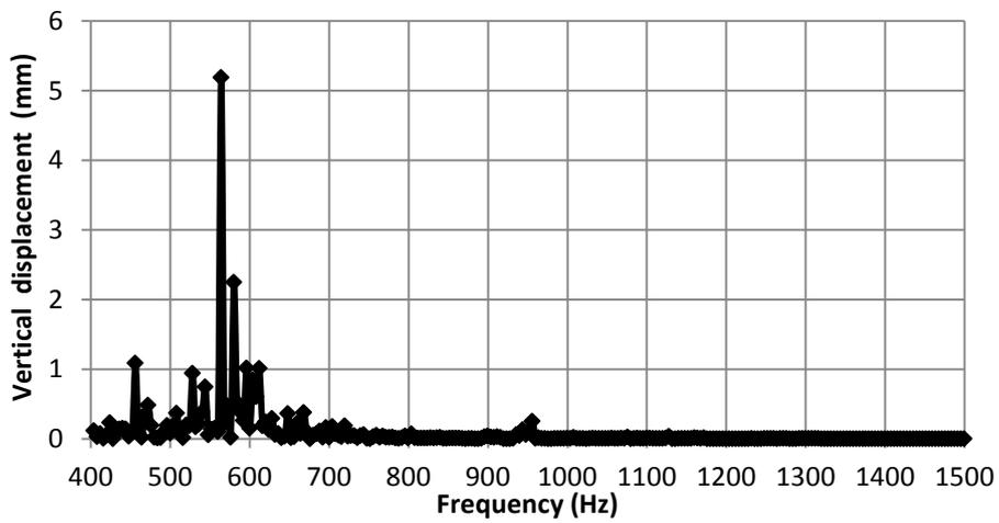
Figure 13. Vertical displacement (at the point of maximum displacement under static loading) due to high harmonic loading range.
