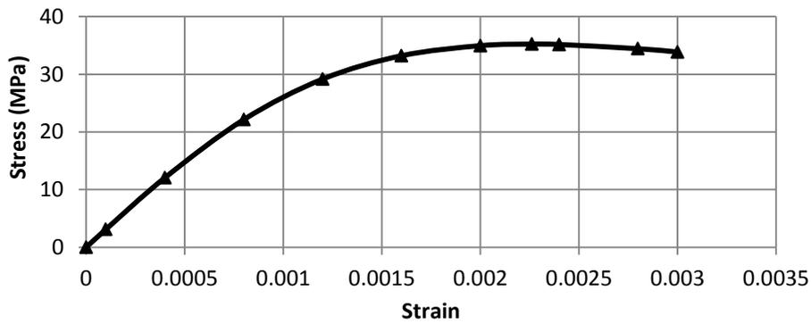
Figure (2). Stress – strain relationship of concrete [1].
