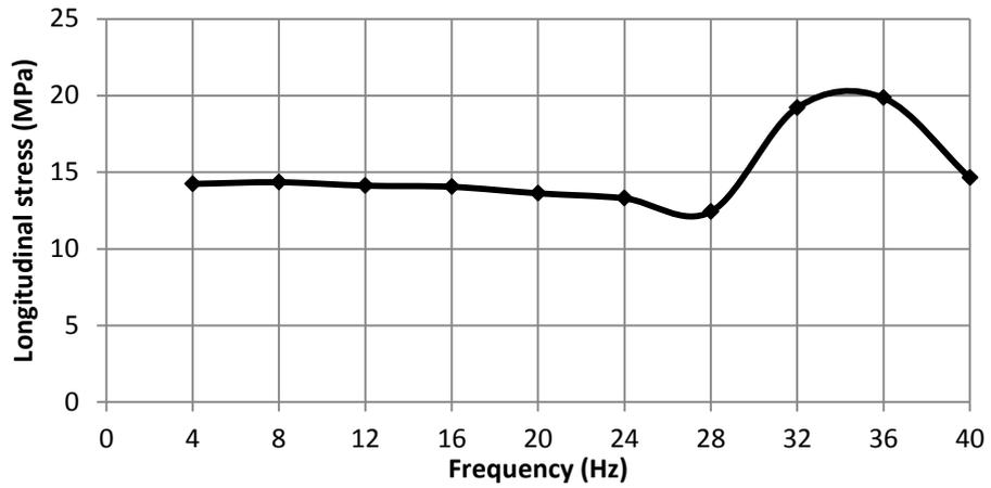
Figure 9. Longitudinal stress of the pile head (node 788) due to low harmonic loading range.
