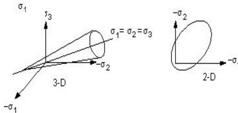
Figure 3. Yield criterion based on Drucker-Prager [15].
