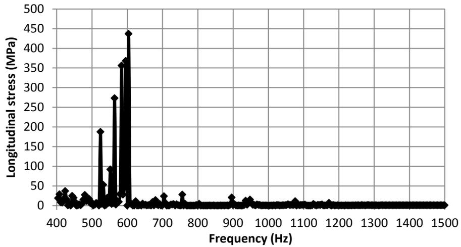
Figure 15. Longitudinal stress of the pile head (node 788) due to high harmonic loading range.
