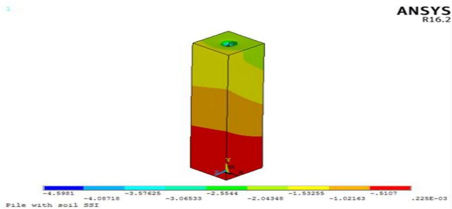
Figure 16. Longitudinal displacement along a pile embedded in soil due to maximum static loading.
