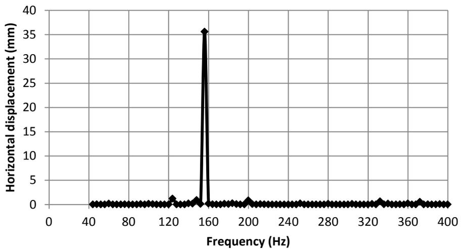
Figure 11. Horizontal displacement of the pile head (node 788) due to medium harmonic loading range.
