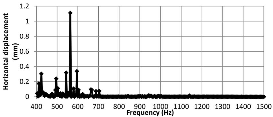
Figure 14. Horizontal displacement of the pile head (node 788) due to high harmonic loading range.
