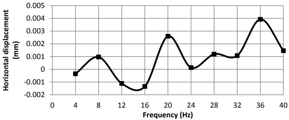
Figure 19. Horizontal displacement of the pile head (node 788) embedded in soil due to low harmonic
