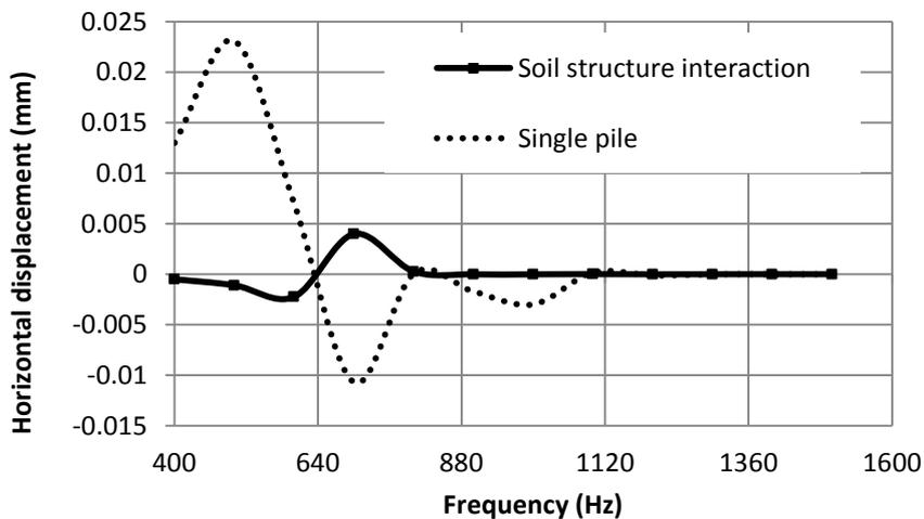
Figure 29. Horizontal displacement of the pile head (node 788) embedded in soil compared with single pile due to high harmonic loading range.
