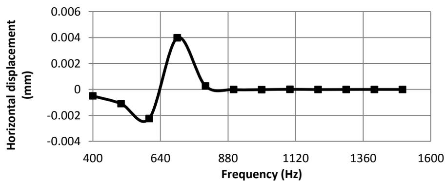
Figure 23. Horizontal displacement of the pile head (node 788) embedded in soil due to high harmonic loading range.
