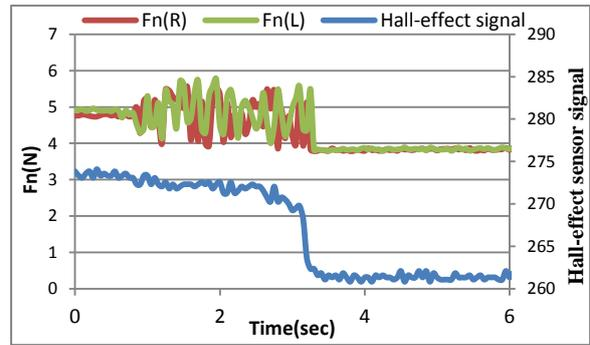
Figure 37. The normal force component with angle slipping 90, glass layer
