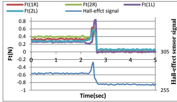
Figure 17. The tangential force component with angle slipping 40, wood layer
