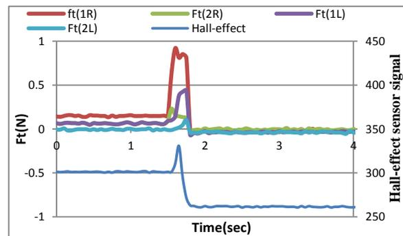
Figure 11. The tangential force component with angle slipping 0, wood layer
