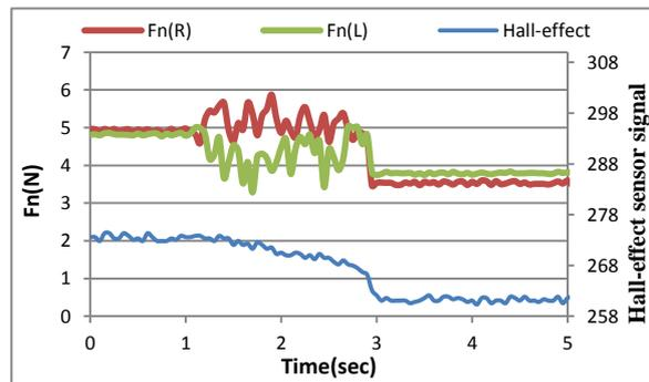
Figure 31. The normal force component with angle slipping 40, glass layer
