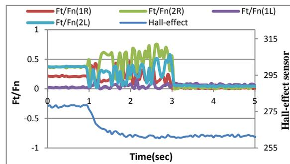
Figure 27. The force ratio with angle slipping 0, wood layer
