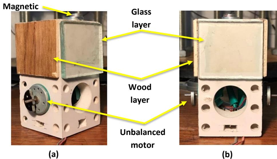
Figure 5. (a) 3D view and (b) side view of experimental object
