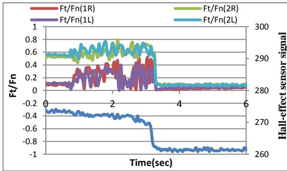
Figure 36. The force ratio with angle slipping 90, glass layer
