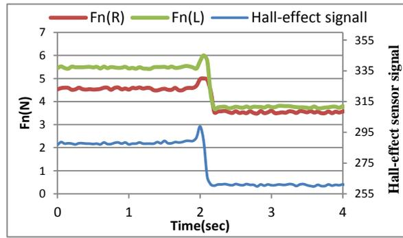
Figure 7. The normal force component with angle slipping 0, glass layer
