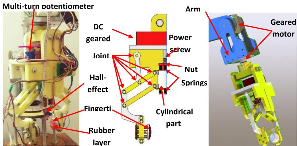
Figure 4. Robotic gripper mechanism
