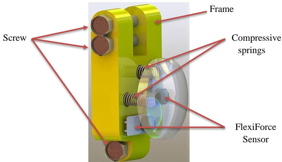
Figure 2. FlexiForce Sensors and Springs Mounting with Fingertip
