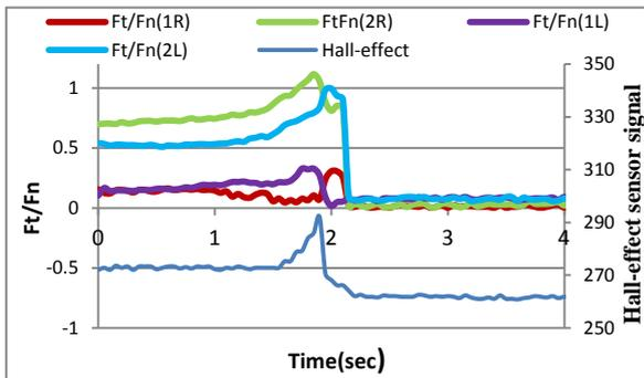
Figure 21. The force ratio with angle slipping 90, wood layer
