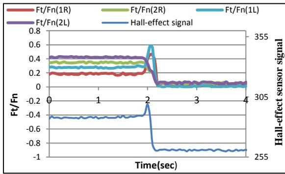
Figure 6. The force ratio with angle slipping 0, glass layer
