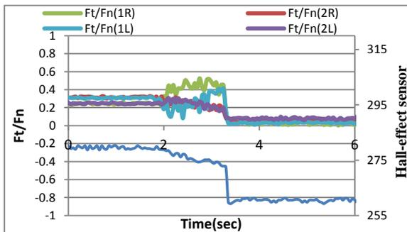
Figure 24. The force ratio with angle slipping 0, glass layer
