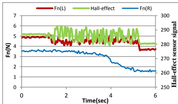
Figure 40. The normal force component with angle slipping 90, glass layer
