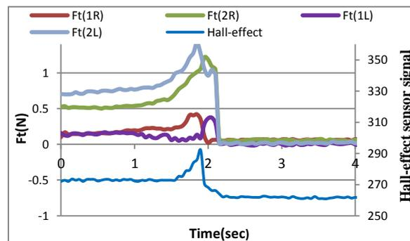
Figure 23. The tangential force component with angle slipping 90, wood layer
