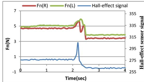
Figure 19. The normal force component with angle slipping 90, glass layer
