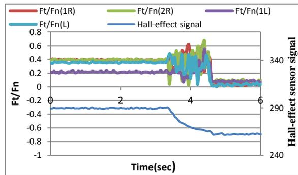
Figure 33. The force ratio with angle slipping 40, wood layer
