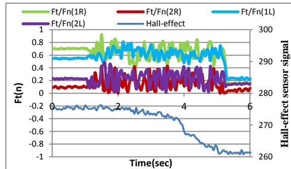
Figure 39. The force ratio with angle slipping 90, wood layer
