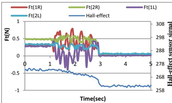
Figure 32. The tangential force component with angle slipping 40, glass layer
