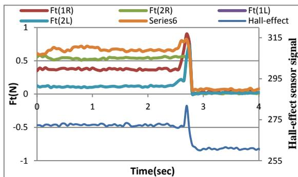
Figure 14. The tangential force component with angle slipping 40, glass layer
