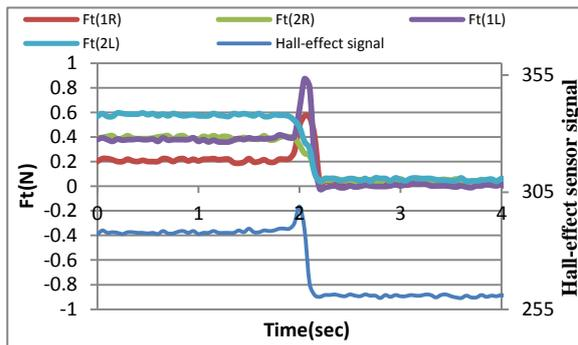
Figure 8. The tangential force component with angle slipping 0, glass layer
