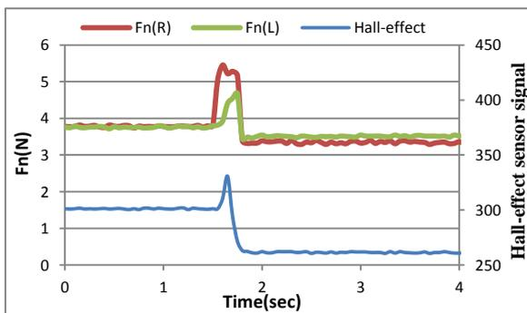
Figure 10. The normal force component with angle slipping 0, wood layer
