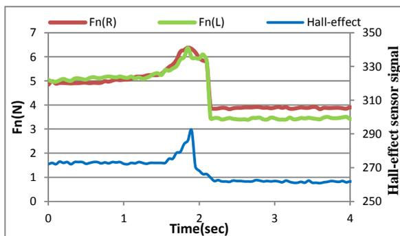
Figure 22. The normal force component with angle slipping 90, wood layer
