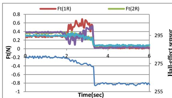
Figure 26. The tangential force component with angle slipping 40, glass layer
