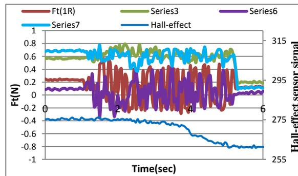
Figure 41. The tangential force component with angle slipping 90, glass layer
