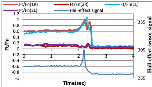
Figure 18. The force ratio with angle slipping 90, glass layer
