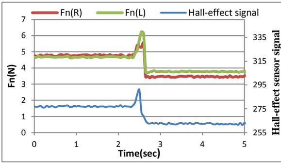
Figure 16. The normal force component with angle slipping 40, wood layer
