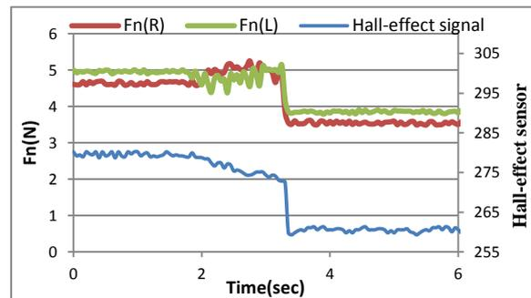
Figure 25. The normal force component with angle slipping 0, glass layer
