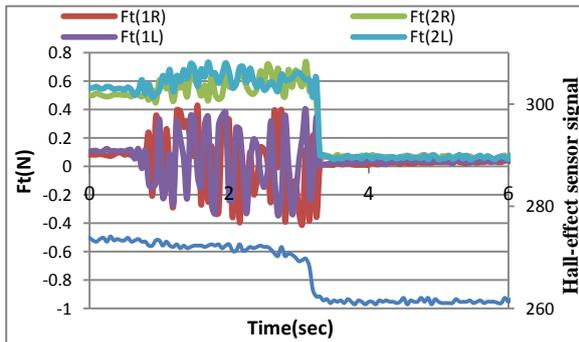
Figure 38. The tangential force component with angle slipping 90, glass layer
