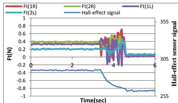
Figure 35. The tangential force component with angle slipping 40, wood layer
