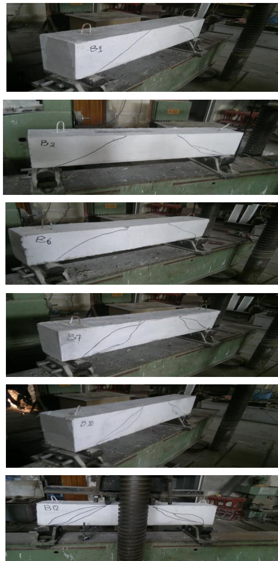
Figure 8. Crack pattern of the tested beam Specimens.
