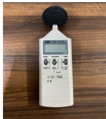
Figure 5. A Sound Level Meter with a wind shield was used in tests.
