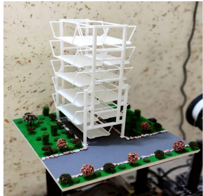
Figure 8. A Prototype of a rotary smart parking system (prepared by the authors of the graduate project for the year 2021-2022).
