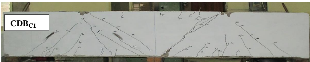
Figure 13. Crack pattern for beam CDB C1 after testing
