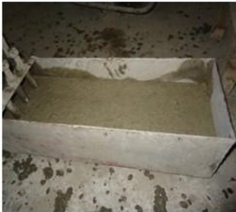
Figure (3-a). Flowing of concrete in horizontal section in L-box test of SCC.
