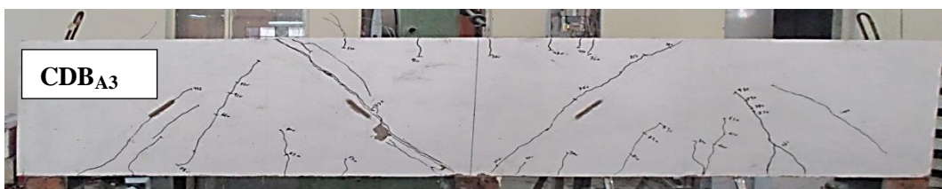
Figure 7. Crack pattern for beam CDB A3 after testing
