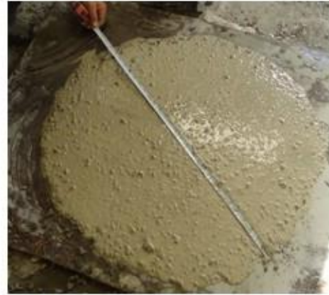
Figure (3-b) Spreading concrete in Slump Flow test of SCC.
