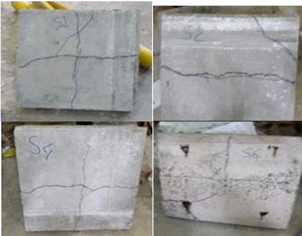
Figure 3. Crack pattern and mode failure for slabs.
