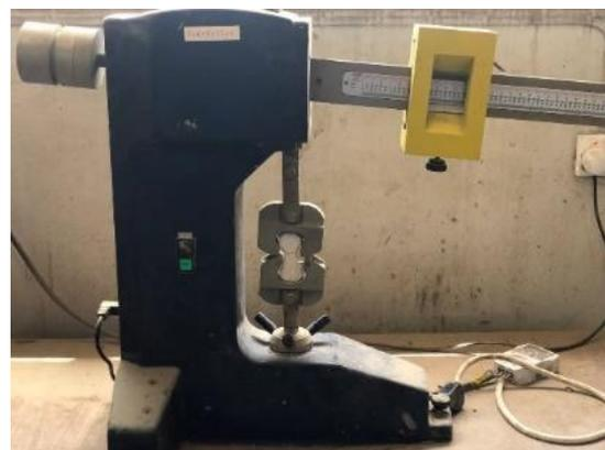
**Figure 4.** Tensile Test Machine
