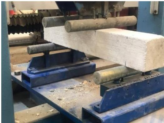
**Figure 5.** Flexural Test for AAC Prism
