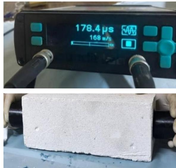
**Figure 3.** Ultrasonic Machine and Test
