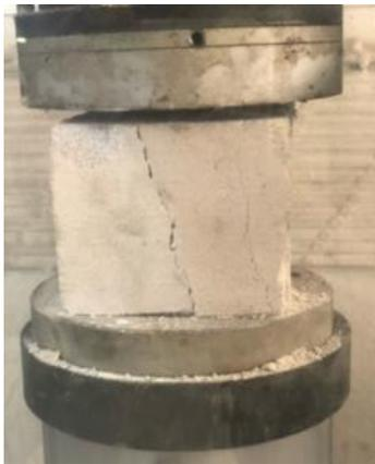
**Figure 2.** Compressive Strength Test for Autoclaved Aerated Concrete Cubic Specimens
