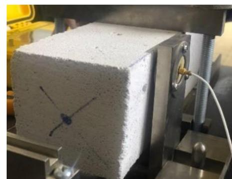
**Figure 8.** Testing of Torsional Resonance Frequency (James Instruments)
