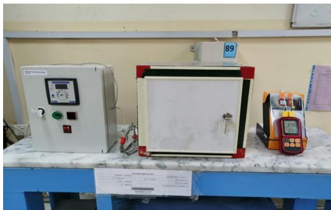
Figure 4. Device used to measure thermal conductivity
