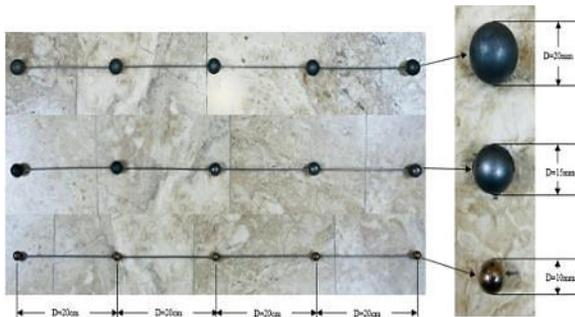
Figure 5. Ball turbulators models and arrangement.
