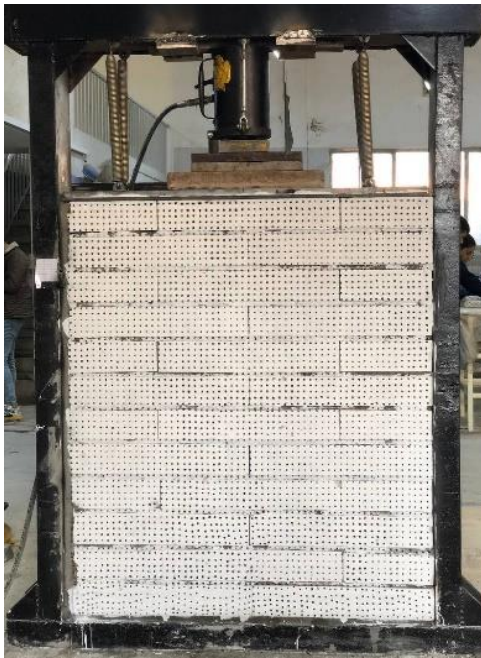
Figure 1. Confined Wall in Steel Frame.
