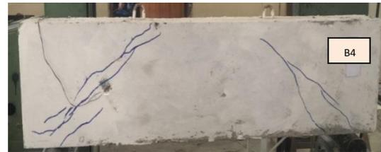
Plate (4) Crack Pattern of Beam4
