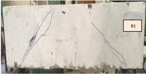
Plate (1) Crack Pattern of Beam1
