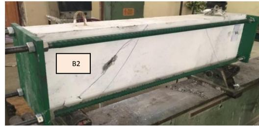
Plate (2) Crack Pattern of Beam2
