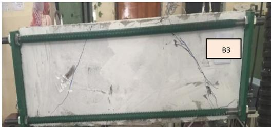
Plate (3) Crack Pattern of Beam3
