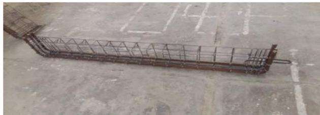
Plate 1. Steel Reinforcement Cage Used for Deep Beams
