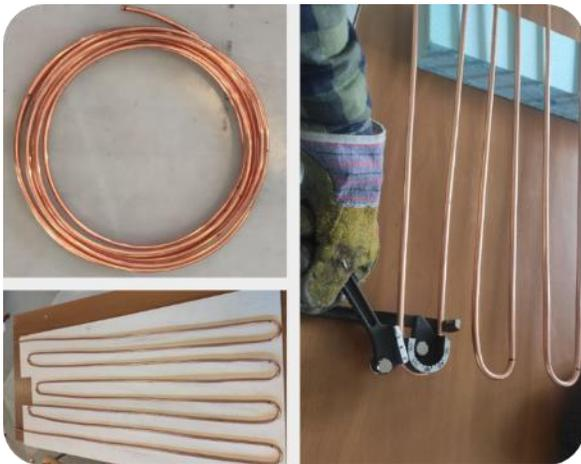
**Figure 1.** Fabrication of the serpentine tube
