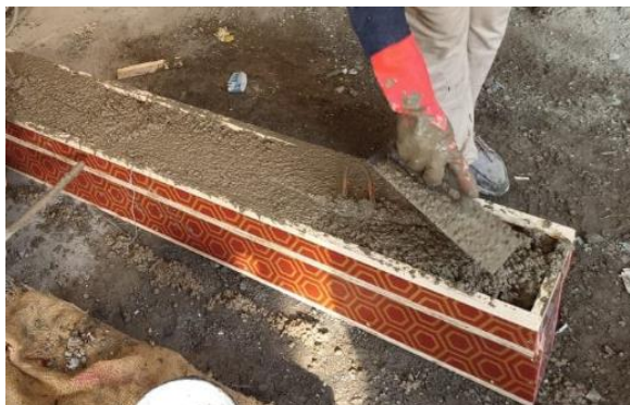
Figure 6. Leveling the casted specimens
