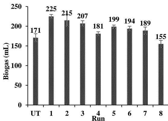
**Figure. 4** Cumulative biogas production of subcritical water pretreated and untreated pineapple waste.
