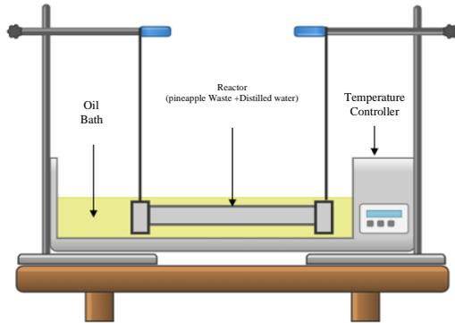
**Figure 1.** Subcritical water pre-treatment setup
