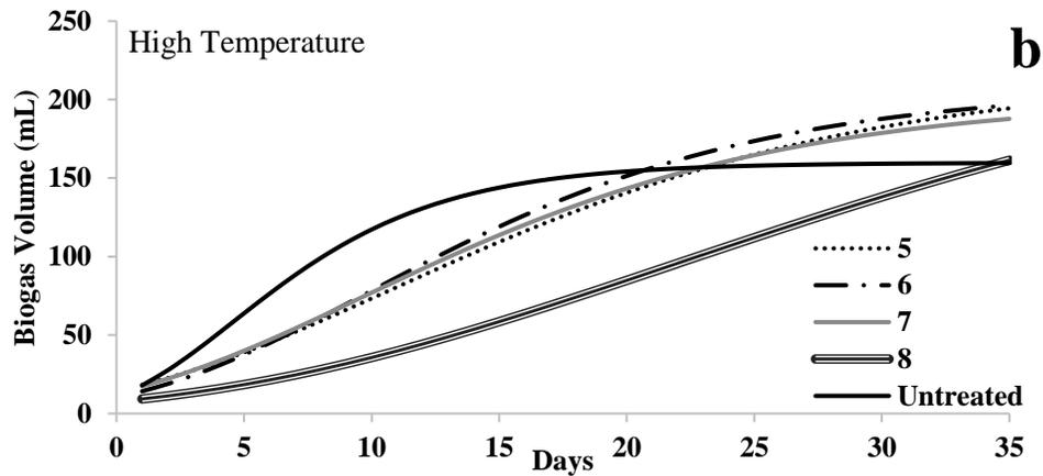
**Figure 6** Comparison of biogas production of subcritical water pretreated pineapple waste using Modified Gompertz model equation (a) Low temperature (120°C) (b) High temperature (200°C).
