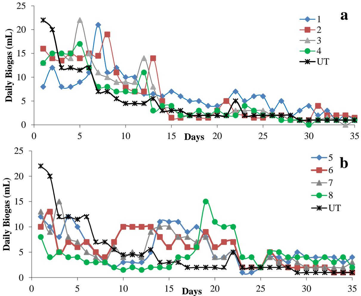
**Figure. 3** Daily biogas production of (a) low temperature (120°C) and (b) high temperature (200°C) of subcritical water pretreated and untreated pineapple waste
