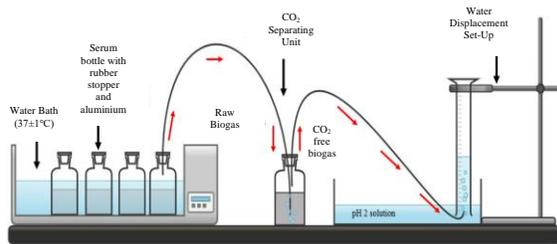
**Figure 2.** Anaerobic digestion set-up
