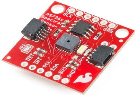
Figure 5. AS7263 NIR Spectral Sensor IC
