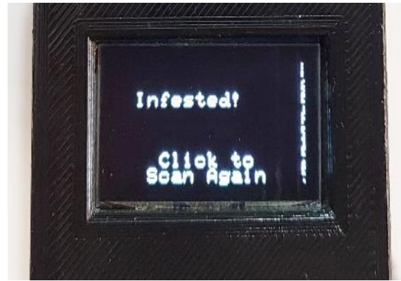
Figure 24. Infested classification result of the prototype
