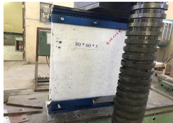
Figure 2. Wall samples under testing
