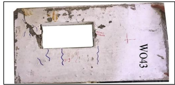
Figure 10. crack pattern of the fourth group
