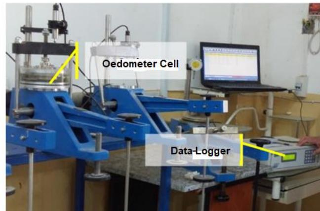
**Figure 1.** Setup of the Computerized Oedometer.
