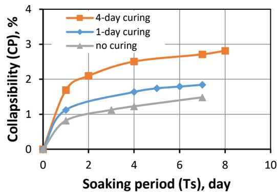
**Figure 8.** Collapse potential (CP) for 12% nanoclay and different curing durations.
