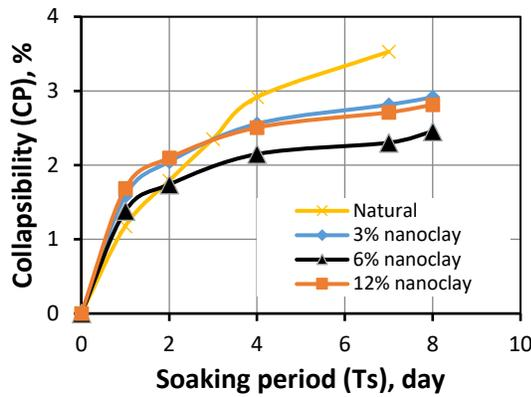
Figure 4. Collapse potential (CP) versus soaking period for 4-day curing.
