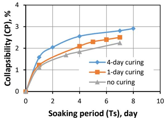
Figure 6. Collapse potential (CP) for 3% nanoclay and different curing durations.
