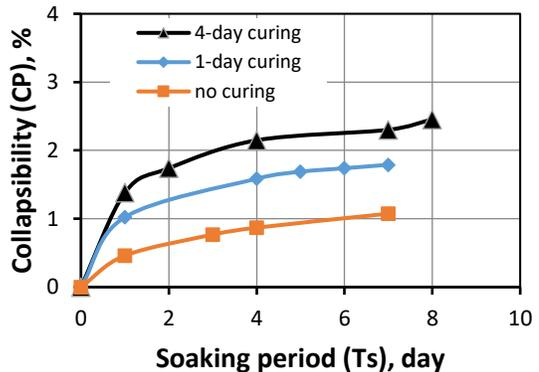
Figure 7. Collapse potential (CP) for 6% nanoclay and different curing durations.
