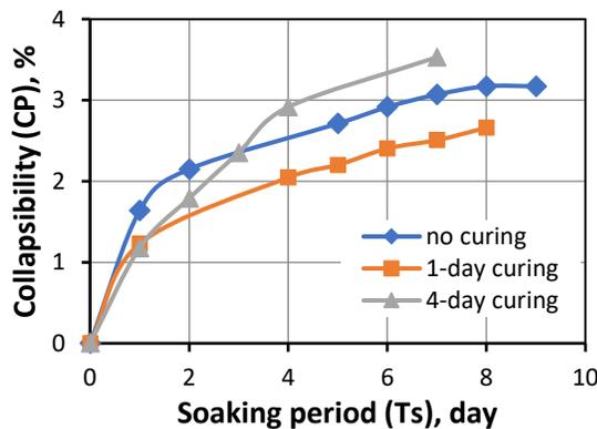
Figure 5. Collapse potential (CP) versus soaking period for no-added soil (natural).
