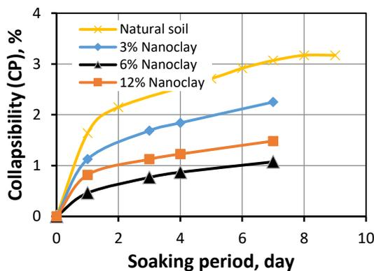
Figure 2. Collapse potential (CP) versus soaking period for no-curing.
