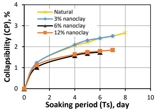
Figure 3. Collapse potential (CP) versus soaking period for 1-day curing.
