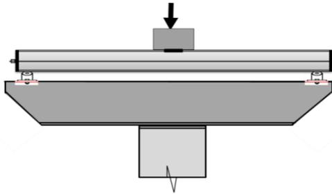
Figure 5. Location of the strain gauges
