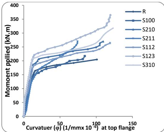
Figure 7. Moment-curvature curves according to the top flange strain
