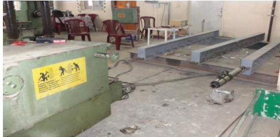
**Figure 3.** The prestressing hydraulic machine
