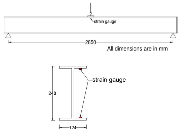
**Figure 4.** Test device, strain gauges, and applied load locations
