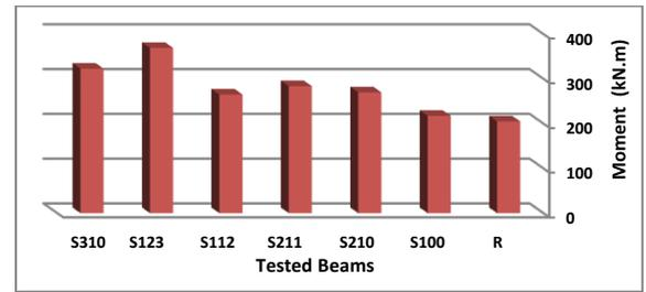
Figure 8. Moment results of tested beams
