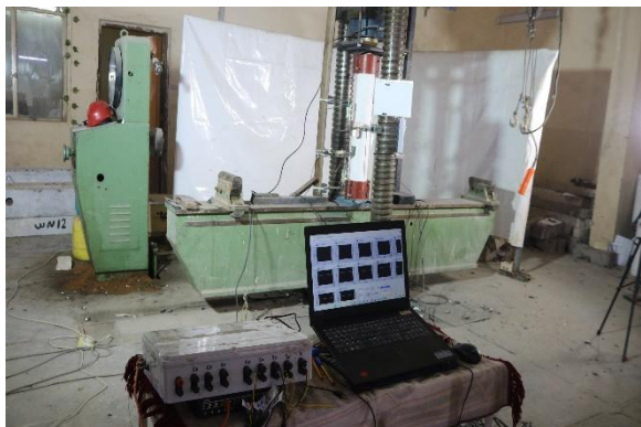
Figure 10. Data logger connected to the computer PC.
