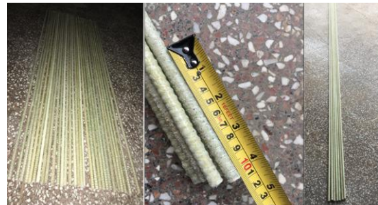
Figure 2. GFRP longitudinal reinforcement.
