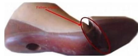
Figure 2. Regions of failure in the SACH foot [7]
