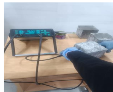
Figure 9. Ultrasonic pulse velocity test
