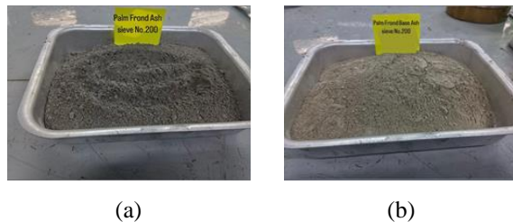
Figure 3. (a) Palm frond ash sieved No. 200 (b) Palm frond base ash sieved No. 200
