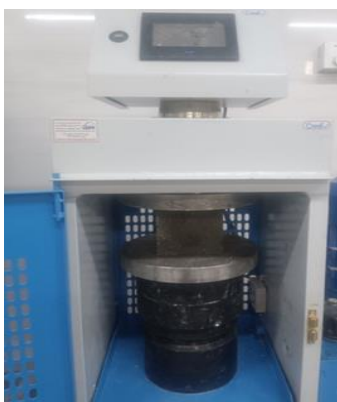
Figure 6. Compressive strength test
