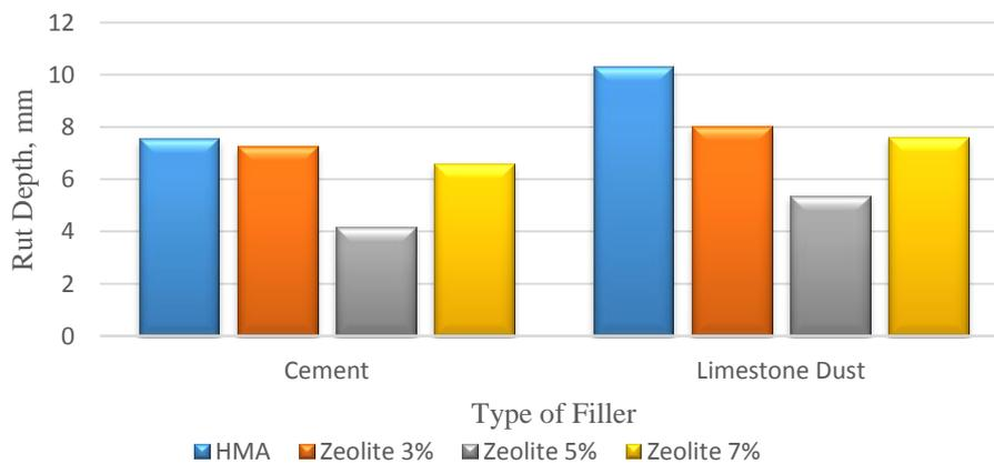
Figure 3. Effect of mix type on rut depth values
