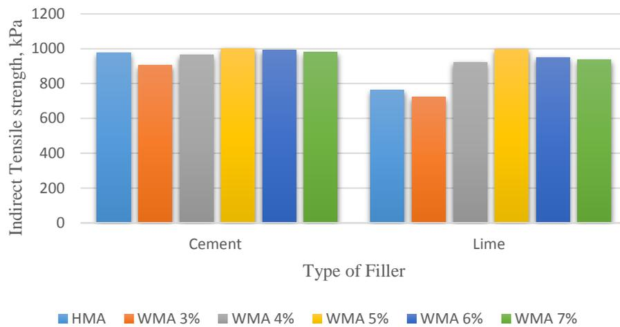
Figure 2. Tensile strength ratio for different asphalt mixtures.
