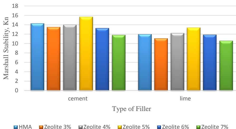
Figure 4. Effect of mix type on Marshall Stability value.
