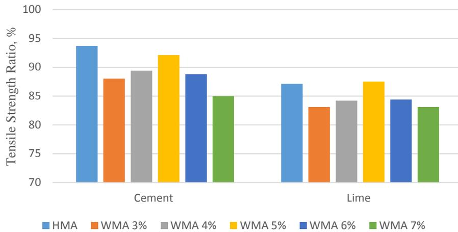
Figure 1. Indirect tensile strength for different asphalt mixtures.
