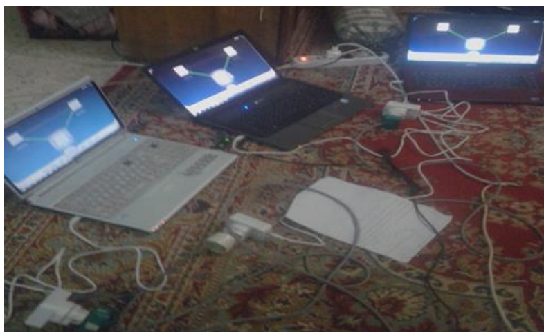
Figure 14. Connect 3 computers with 3 modems used in PLC
