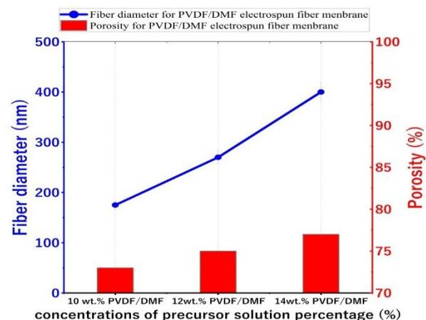
**Figure 5.** The porosity and fiber diameter of the electrospun PVDF nanofiber membranes were investigated at different precursor solution concentrations
