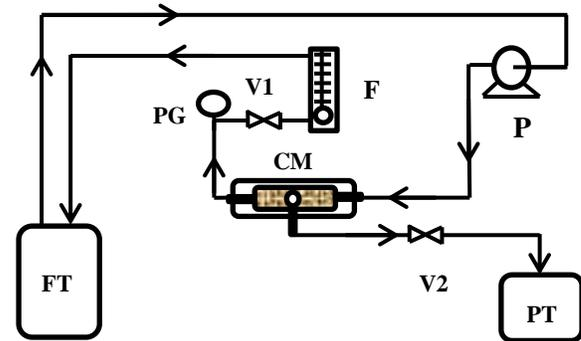
**Figure 1.** Graphical depiction of the crossflow filtration system implemented in the verified study.
