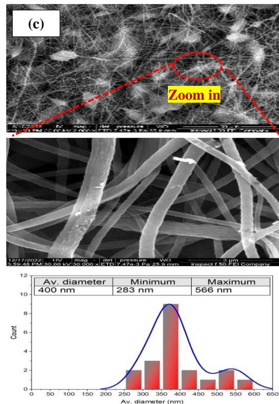
**Figure 2.** The FE-SEM image shows the different precursor concentrations and corresponding fiber diameters: (a) 10 wt.%, (b) 12 wt.%, and (c) 14 wt.% of a PVDF solution in DMF solvent mixture.
