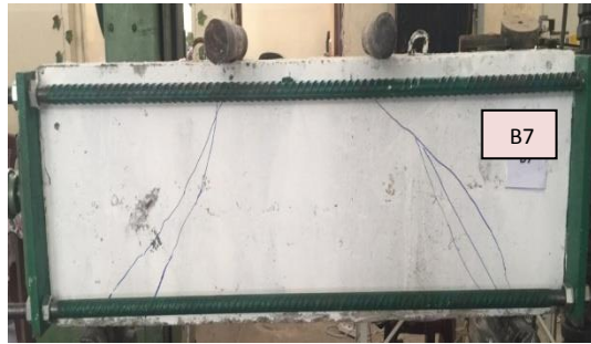
Plate 11. Crack Pattern of Beam 7.
