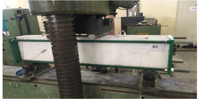
Plate (4) Beam Applied to Two Point Load
