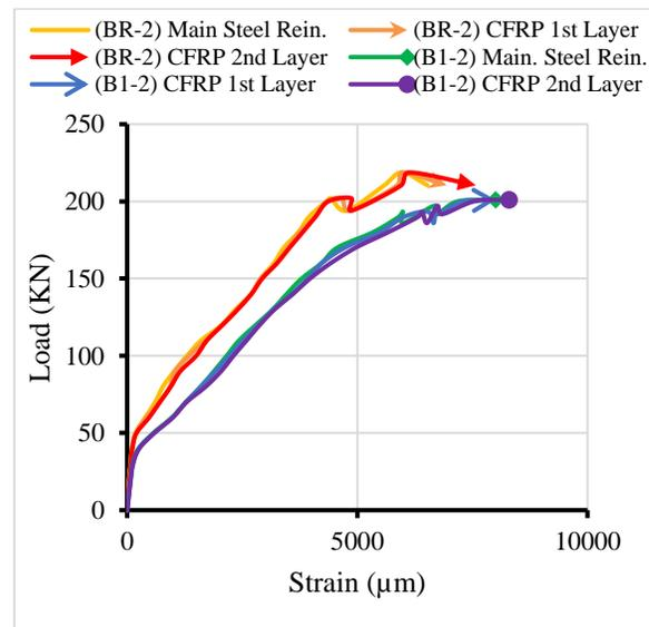
**Figure 17.** The load-strain diagram for the beams (BR-2) and (B1-2)'s main steel reinforcement and CFRP sheet
