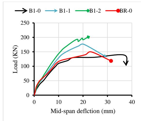
**Figure 14.** Load-deflection diagram of group (B1) beams and (BR-0)
