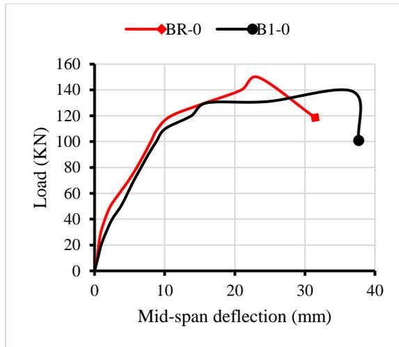
**Figure 11.** Load-deflection diagram for beams (BR-0) and (B1-0)
