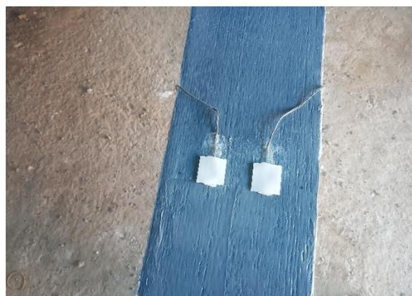
**Figure 5.** Strain gauges are being installed on sheets of (CFRP).
