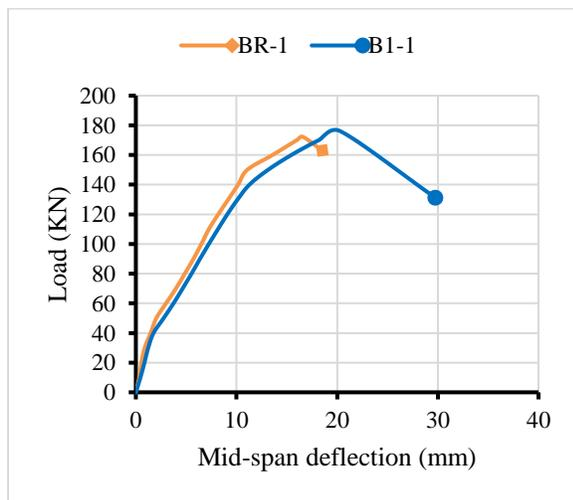
**Figure 12.** Load-deflection diagram of the beams (BR-1) and (B1-1)
