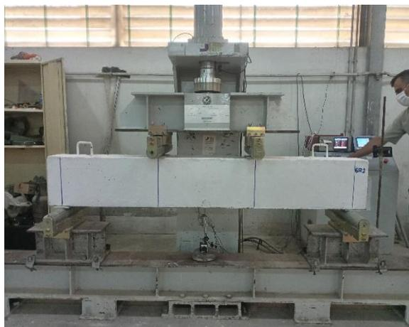
Figure 6. Beam Specimens Set-up
