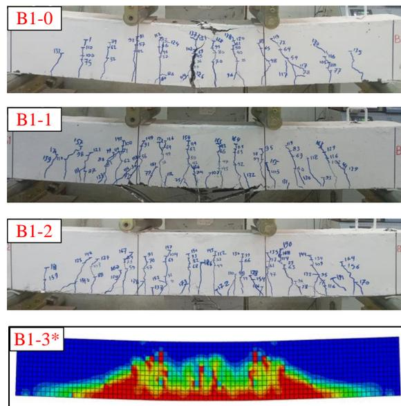
**Figure 8.** Flexural test of the group (B1) beams, B1-0, B1-1, B1-2, and B1-3\* (\*= Numerically representation by finite element analysis)
