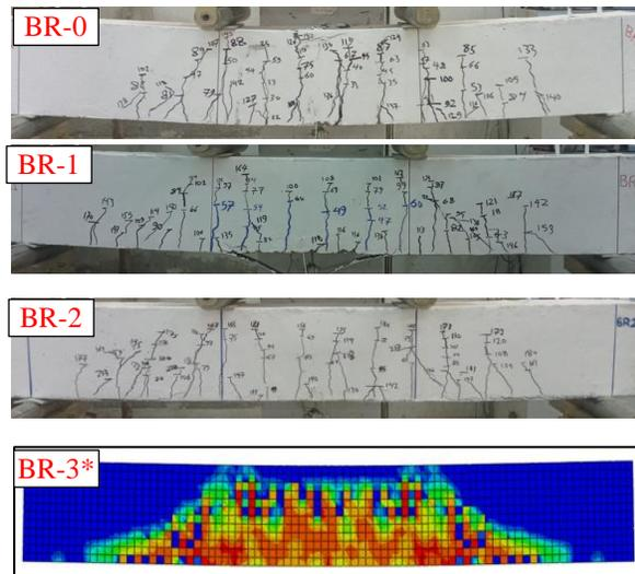
**Figure 7.** Flexural test of the group (BR) beams, BR-0, BR-1, BR-2, and BR-3\*
