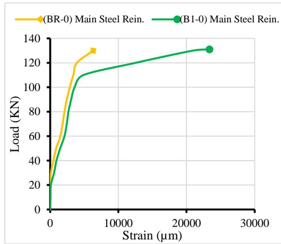
**Figure 15.** Beams (BR-0) and (B1-0) main steel reinforcement load-strain diagram
