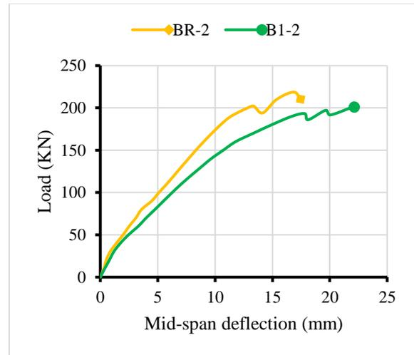
**Figure 13.** Load-deflection diagram of the beams (BR-2) and (B1-2)
