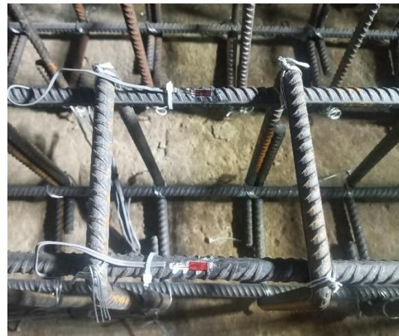
**Figure 4.** Strain gauges are being installed on the main reinforcement.
