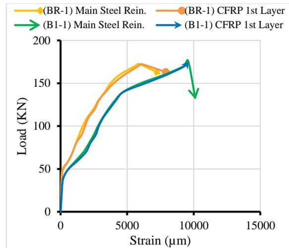
**Figure 16.** load-strain diagram for beams (BR-1) and (B1-1)'s main steel reinforcement and CFRP sheet
