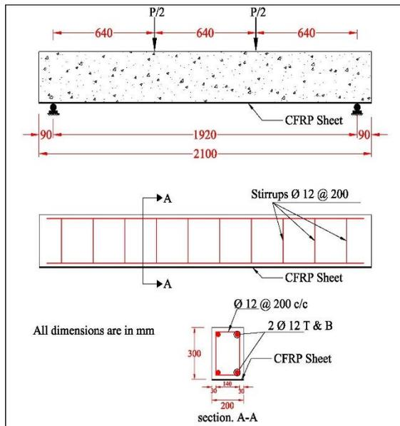
**Figure 1.** Details of the Tested Beam Specimens
