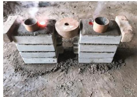
**Figure 2.** Production of specimens by sand casting in sand casting foundry
