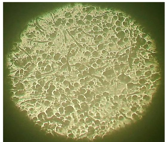
**Figure 12.** Pearlitic ductile iron as-cast. Graphite nodules (spherulites) in the envelopes of free ferrite (bull's-eye structure), in a matrix of pearlite [11]
