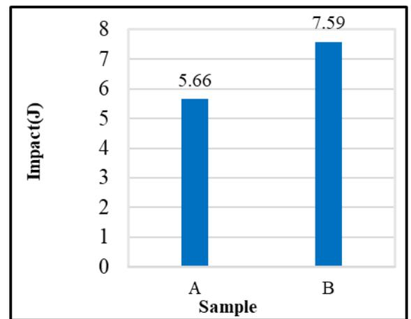
Figure 10. Change of the Charpy impact of samples
