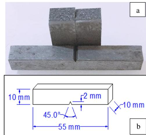
**Figure 4.** Standard Charpy impact specimen: (a) Charpy specimen before and after testing and (b) A schematic of standard Charpy impact
