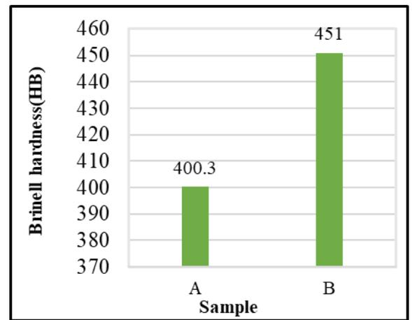
Figure 9. Change of the Brinell hardness of samples
