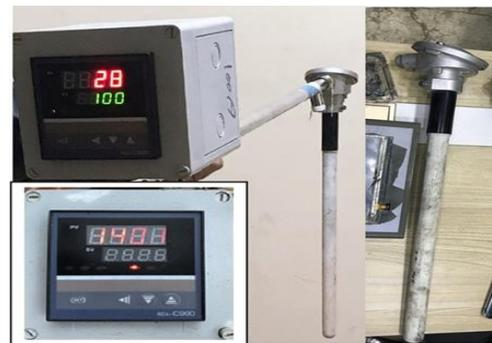
**Figure 1.** Thermocouple type S class 1 (Pt10%Rh-Pt) with temperature controller to monitor the temperature.
