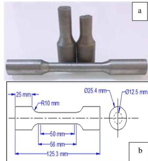
**Figure 3.** Standard tensile specimen: (a) tensile specimen before and after testing and (b) A schematic of standard tensile sample.
