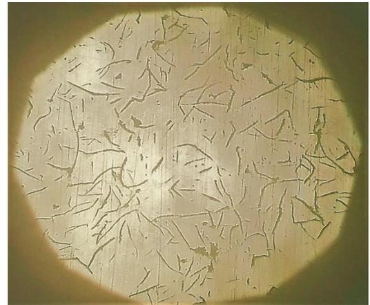
**Figure 11.** Gray cast iron flake graphite in matrix of fine pearlite with less than 10% free ferrite [11]
