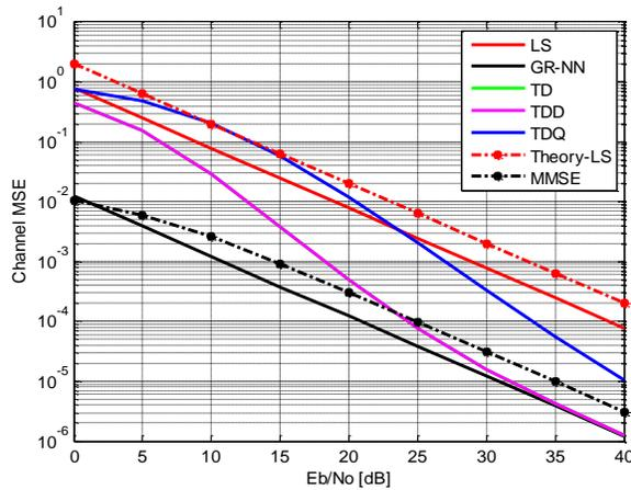
Figure 6. MSE characteristics for size of FFT=64 for 32 QAM
