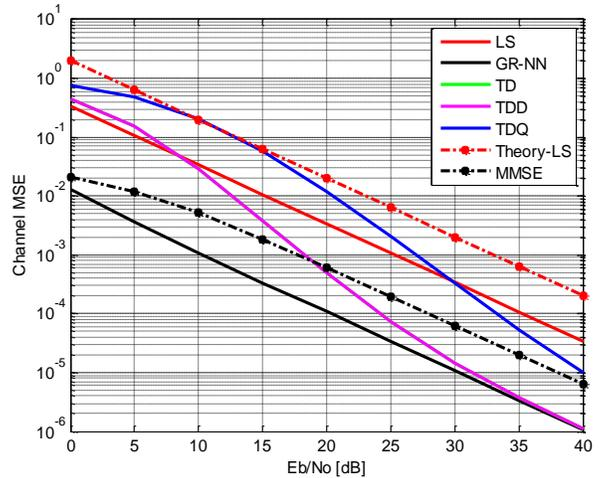
Figure 7. MSE characteristics for size of FFT=32 for 64 QAM
