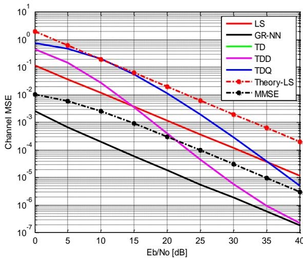
Figure 10. MSE characteristics for the size of FFT=64 for 64 QAM and CP=12
