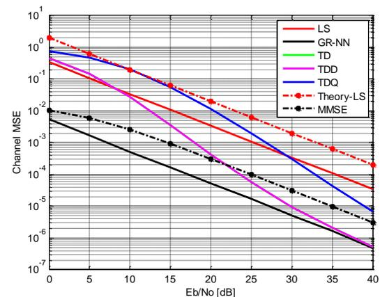
**Figure 5.** MSE characteristics for size of FFT=64 for 16 QAM
