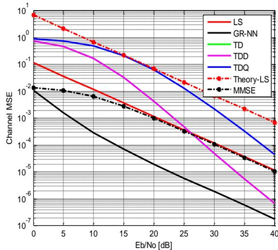
**Figure 12.** MSE characteristics for size of FFT=64 for 64 QAM and  $\beta=2$
