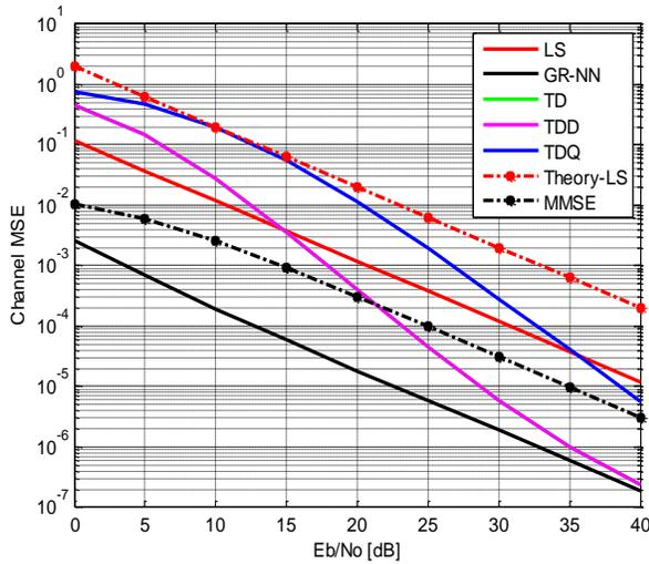
Figure 9. MSE characteristics for size of FFT=64 for 64 QAM and CP=4
