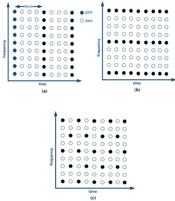
**Figure 4.** Channel estimation Pilot methods: (a) Block-type. (b) Comb-type. (c) Scattered type.
