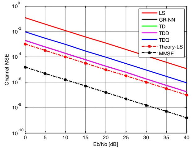
Figure 11. MSE characteristics for size of FFT=64 for 64 QAM and  $\beta=0.001$
