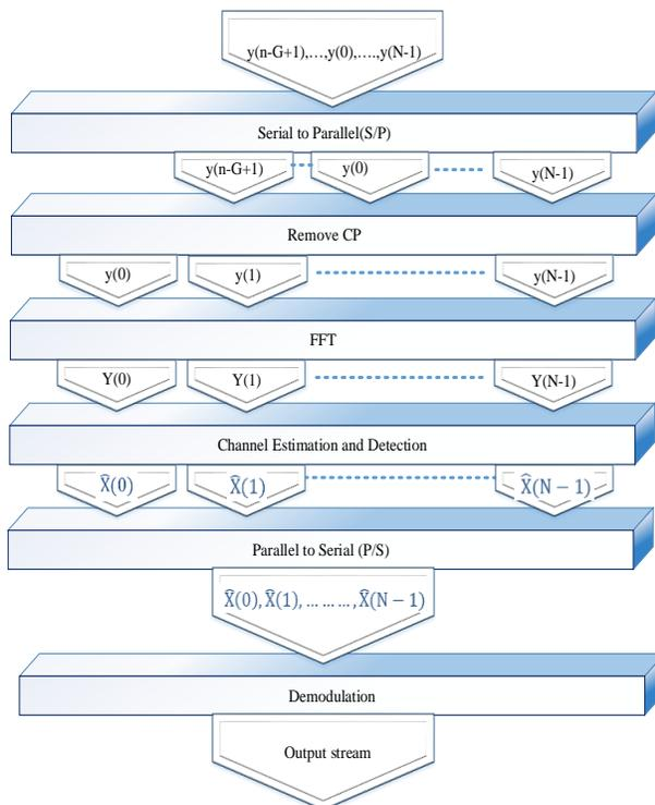
Figure 3. M-QAM OFDM Receiver flowchart.
