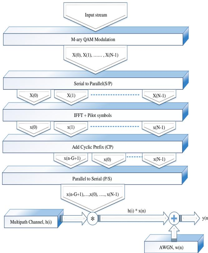
Figure 2. M-QAM OFDM Transmitter flowchart.
