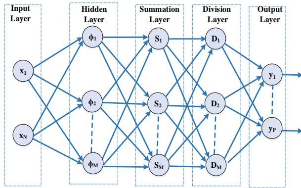
**Figure 1.** Generalized Regression Neural Network (GRNN) architecture.
