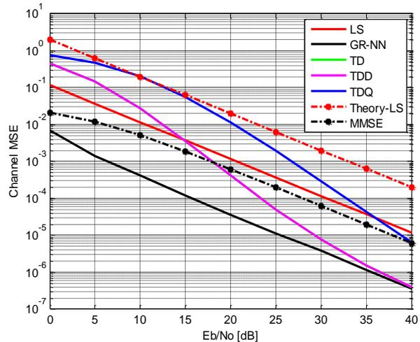
Figure 8. MSE characteristics for size of FFT=64 for 64 QAM
