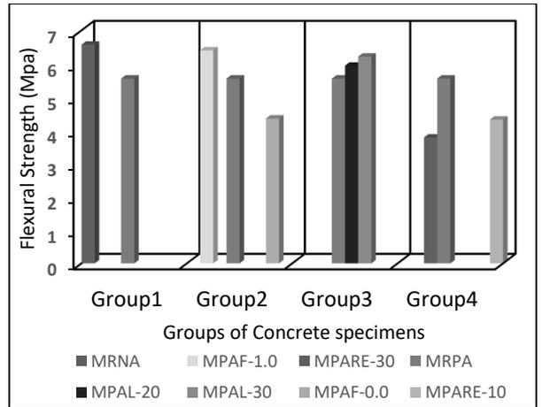
Figure 7. Results of Flexural Strength for All Concrete Specimens.
