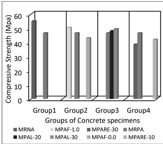
Figure 5. Results of Compressive Strength for All Concrete Specimens
