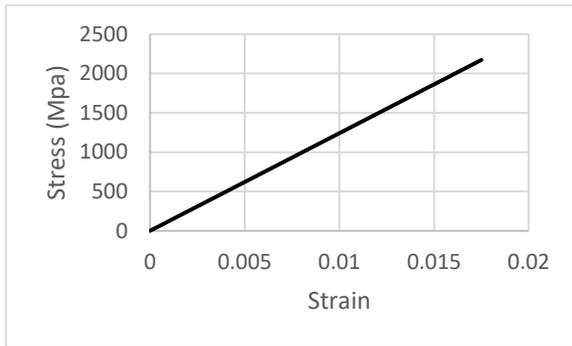
Figure 4. Stress-strain CFRP bar curve
