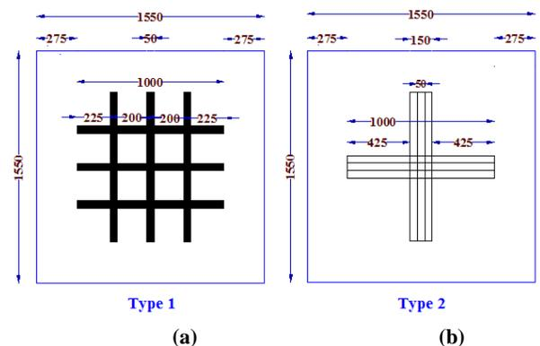
**Figure 1.** CFRP laminates layout- (a) Type 1, (b) Type 2
