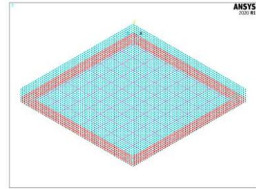
Figure 6. Reinforcement distribution and CFRP laminates layout of model SC
