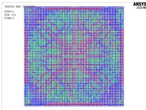
(b) Cracks propagations
