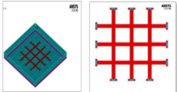
Figure 7. Reinforcement distribution and laminated CFRP layout of model SC1-S1
