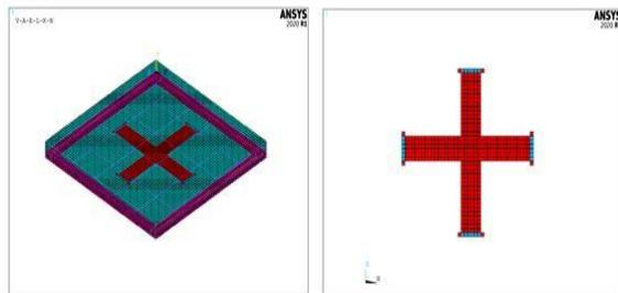
Figure 10. CFRP layout of model SC2-S2-three-dimensions
