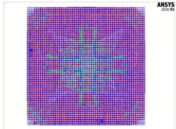
Figure14. Deflection and cracks propagations of model SC1-S2 at final stage analysis
