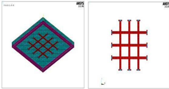
Figure 9. Reinforcement's distribution and CFRP layout of model SC2-S1
