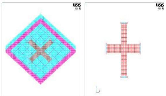
Figure 8. Reinforcement distribution and CFRP layout of model SC1-S2
