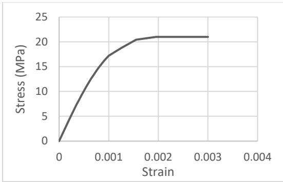
Figure 2. Stress-strain curve concrete of compression
