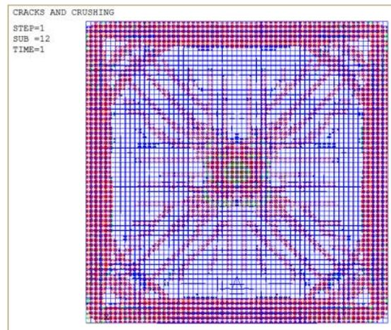
(b) Cracks Propagations
