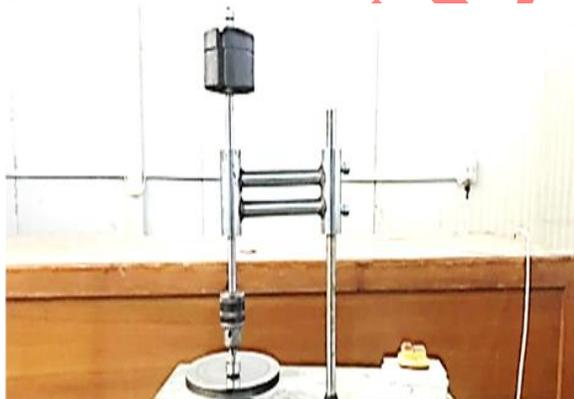
**Figure 7.** A pin-on-disk device is a common tool for wear testing.
