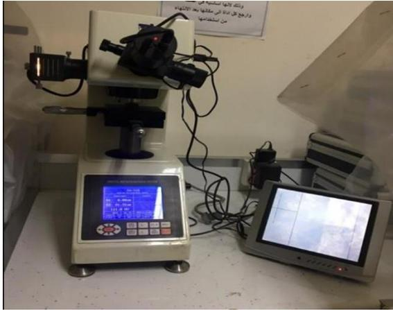
**Figure 6.** A Digital Micro Hardness Device.
