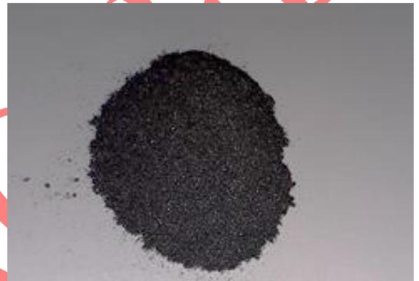
**Figure 3.** Graphite powder that gives the sample surface some roughness.
