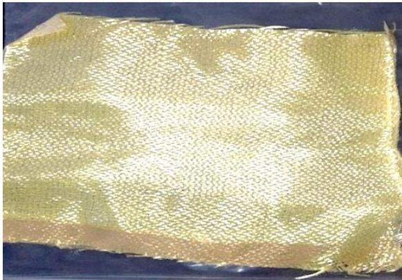
**Figure 1.** The design and manufacturing of Kevlar fiber. The Kevlar fiber (aramid 49 type) properties are shown in Table 1.
