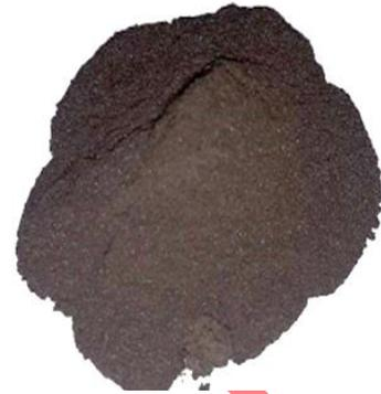
**Figure 2.** Pure iron powder used to make castings.
