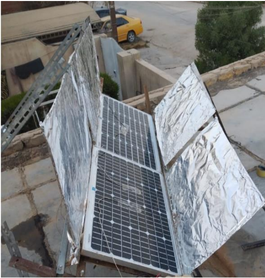
Figure 2. Experimental photovoltaic concentration rig with PCM and fins.
