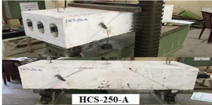
Plate (8) Crack Pattern for HCS-250-A
