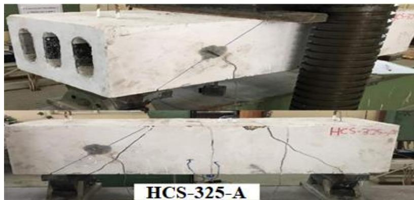
Plate (9) Crack Pattern for HCS-325-A
