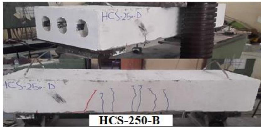
Plate (11) Crack Pattern for HCS-250-B
