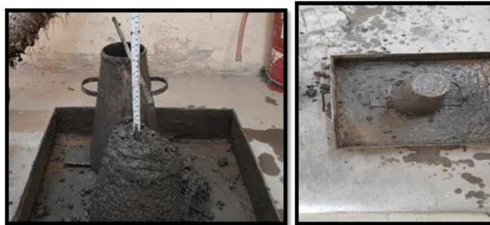
Plate (6) Slump Test
