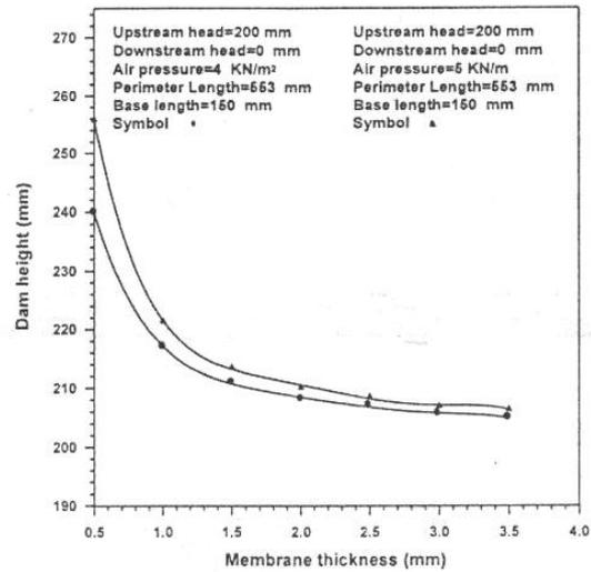
Fig.25 Variation of Dam Height with Membrane Thickness (Air-inflated Dam)
