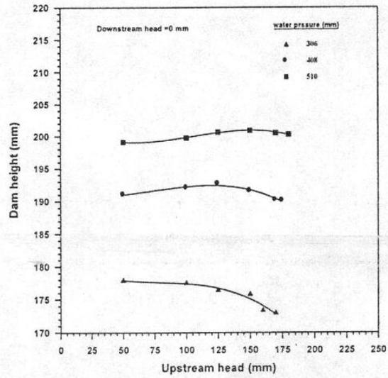
Fig. 11 Variation of Dam Height with Rising Upstream Head for Various Water Pressures.
