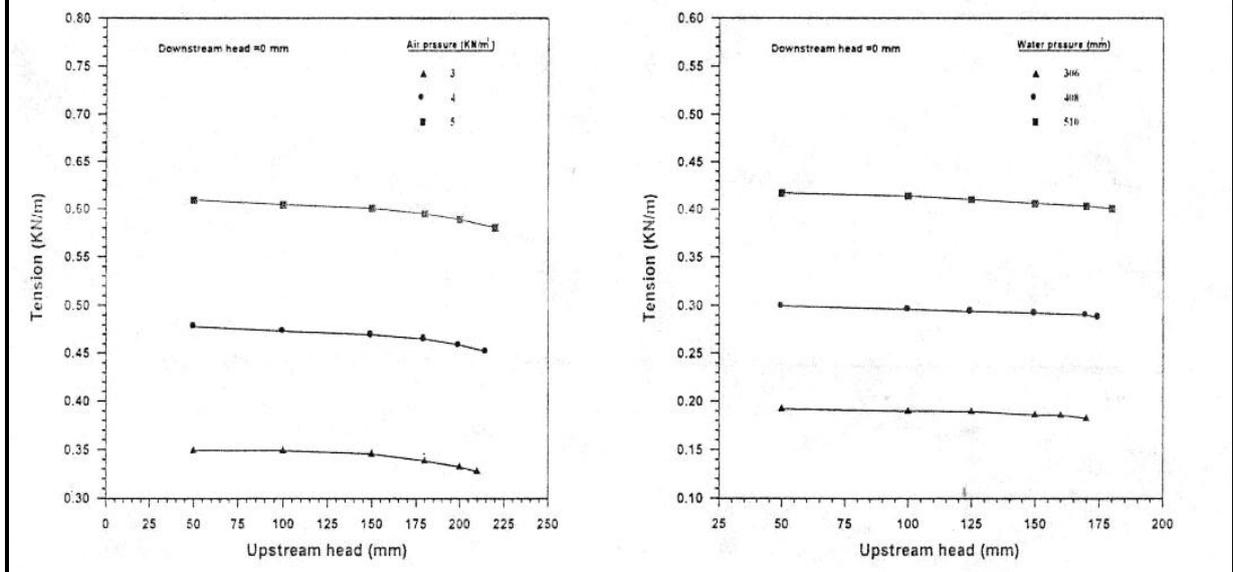
Fig. 8 Variation of Membrane Tension with Rising Upstream Head for Various Air Pressures.
