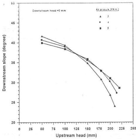
Fig.14 Variation of Membrane Slope at Downstream Fixture for Rising Upstream Head and Various Air Pressures.
