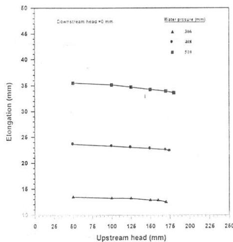
Fig.19 Variation of Elongation in Membrane for Rising Upstream Head and Various Water Pressures.
