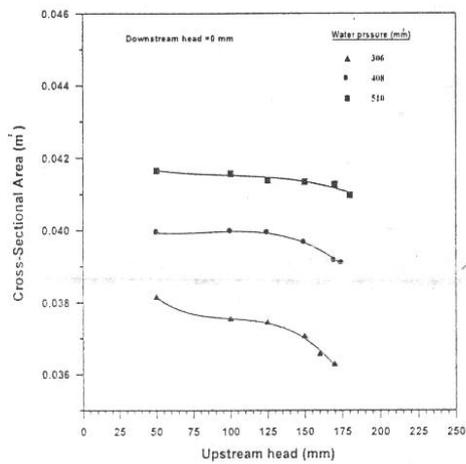
Fig.17 Variation of Dam Cross-sectional Area for Rising Upstream Head and Various Water Pressures.
