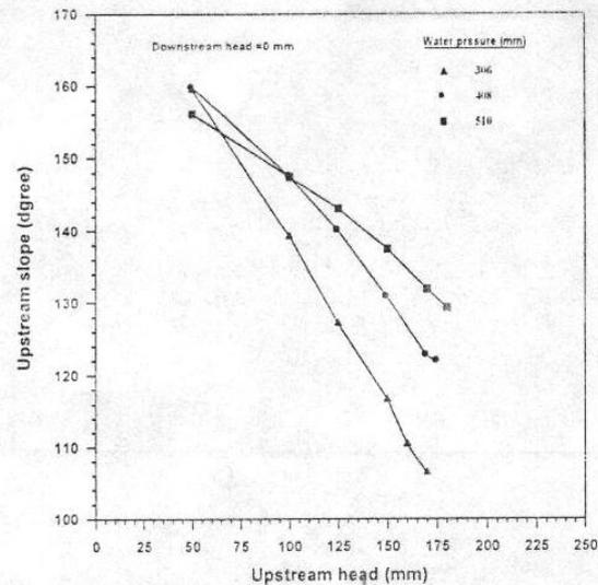
Fig.13 Variation of Membrane Slope at Upstream Fixture for Rising Upstream Head and Various Water Pressures.
