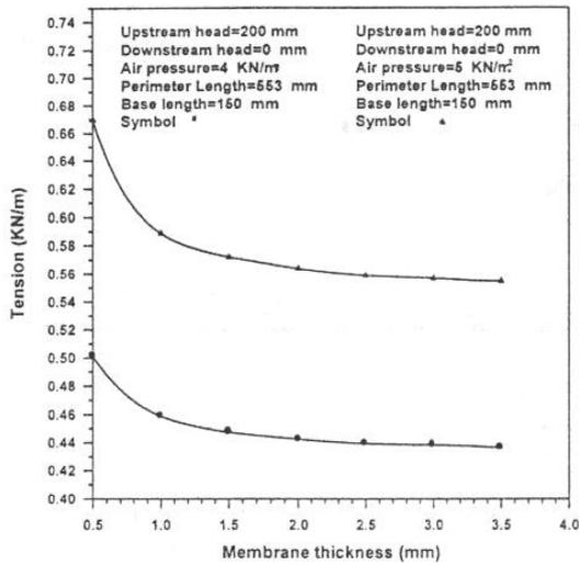
Fig.24 Variation of Membrane Tension with Membrane Thickness (Air-inflated Dam)
