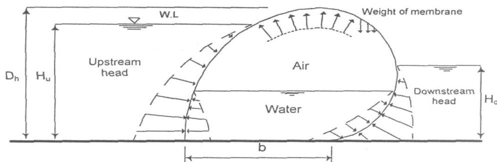
**Figure (1) Forces Acting on the Dam (Hydrostatic Condition)**
