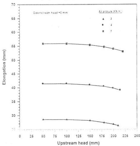
Fig.18 Variation of Elongation in Membrane for Rising Upstream Head and Various Air Pressures.
