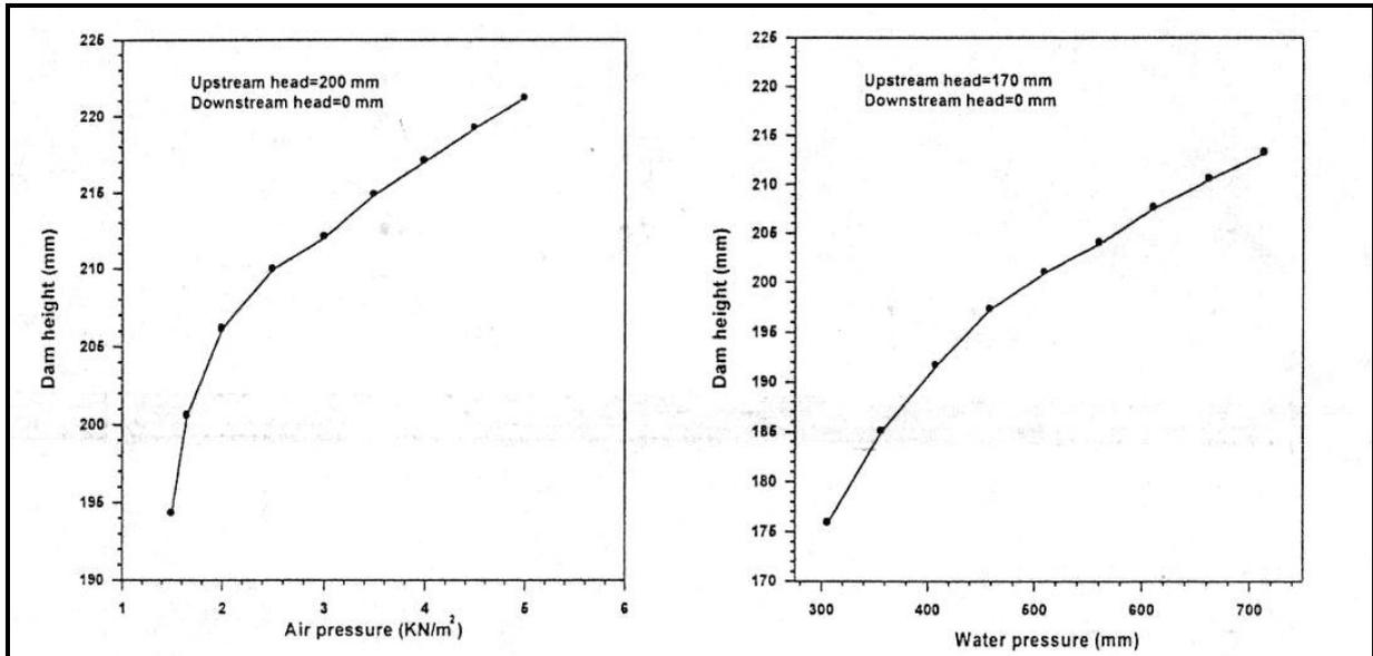
Fig.6 Variation of Dam Height with Increasing Internal Air Pressure for Constant Upstream Head and Downstream Head
