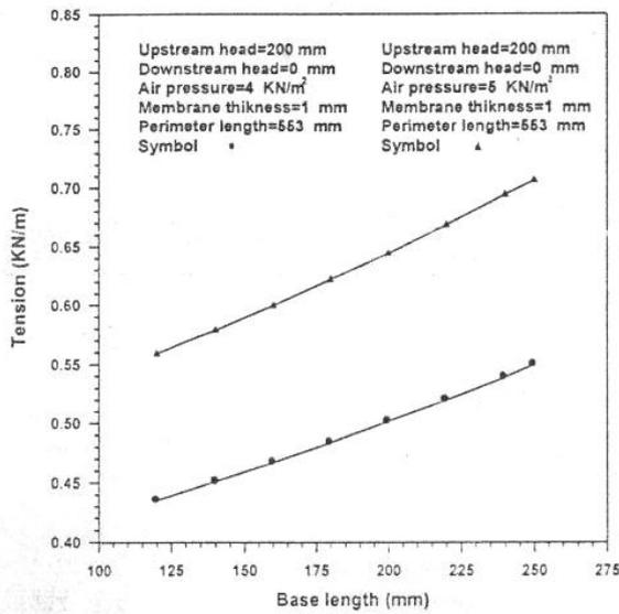
Fig.28 Variation of Membrane Tension with Base Length of the Dam (Air-inflated Dam)
