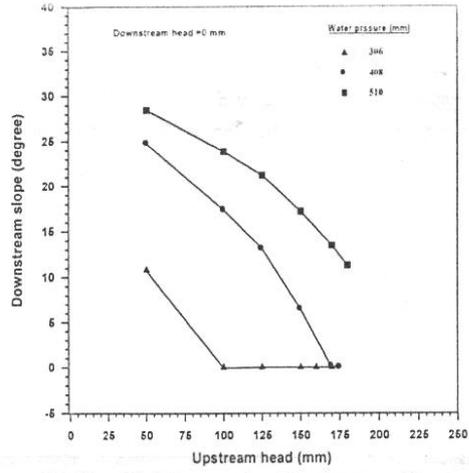
Fig.15 Variation of Membrane Slope at Downstream Fixture for Rising Upstream Head and Various Water Pressures.
