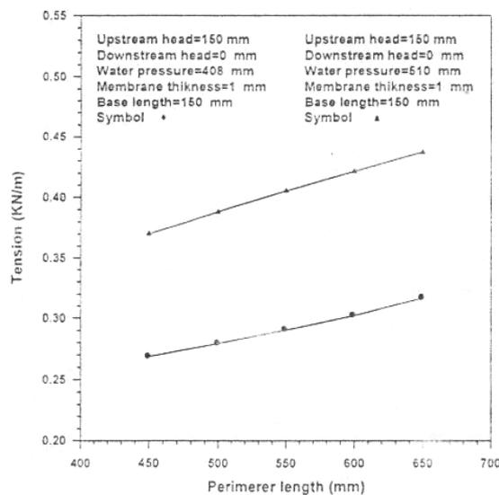
Fig.22 Variation of Membrane Tension with Membrane Perimeter Length (Water-inflated Dam)
