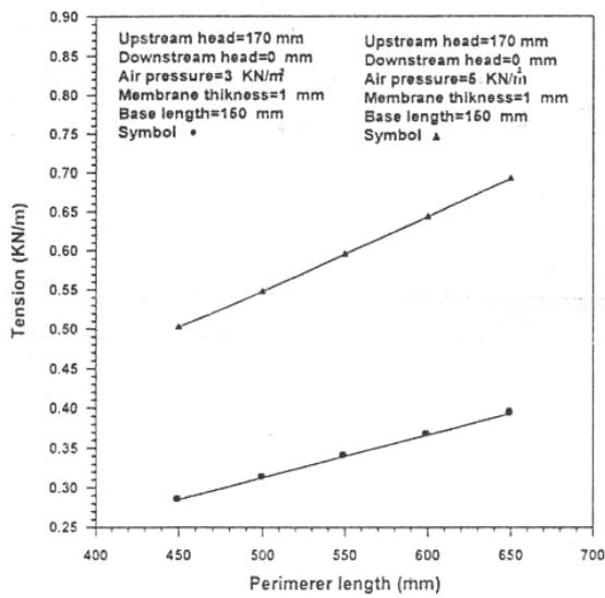
Fig.20 Variation of Membrane Tension with Membrane Perimeter Length (Air-inflated Dam)
