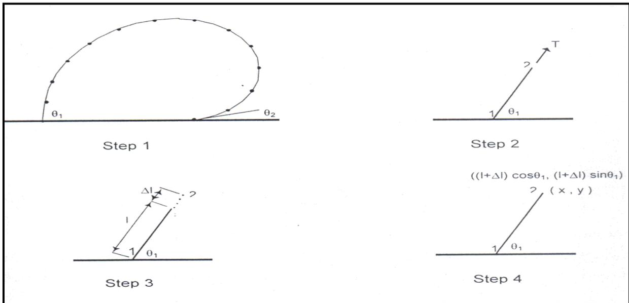
Figure (A-2) Co-ordinates of Nodes of the Dam Profile
