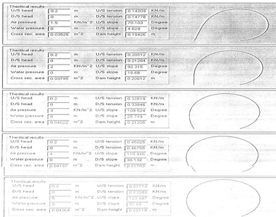
Figure (4) Effect of Increasing Internal Pressure on the Behavior of Air-Inflated Dams for Constant Upstream Head and Downstream Head
