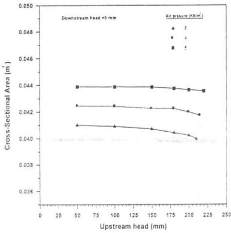
Fig.16 Variation of Dam Cross-sectional Area for Rising Upstream Head and Various Air Pressures.
