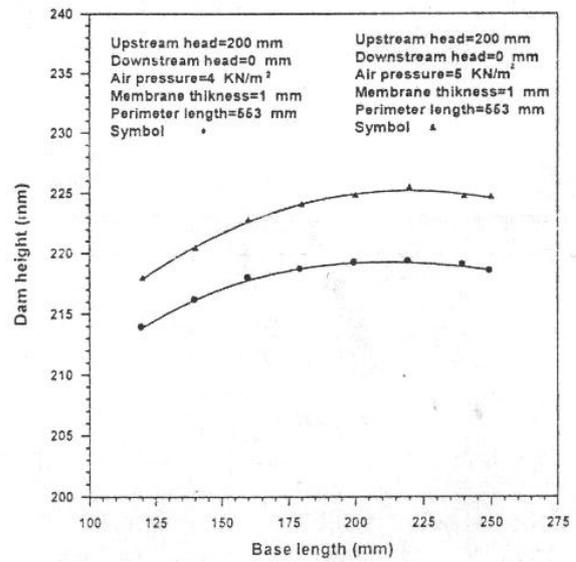
Fig.29 Variation of Dam Height with Base Length of the Dam (Air-inflated Dam)
