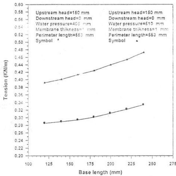
Fig.30 Variation of Membrane Tension with Base Length of the Dam (Water-inflated Dam)
