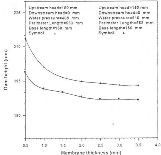
Fig.27 Variation of Dam Height with Membrane Thickness (Water-inflated Dam)
