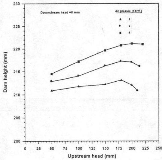
Fig. 10 Variation of Dam Height with Rising Upstream Head for Various Air Pressures.
