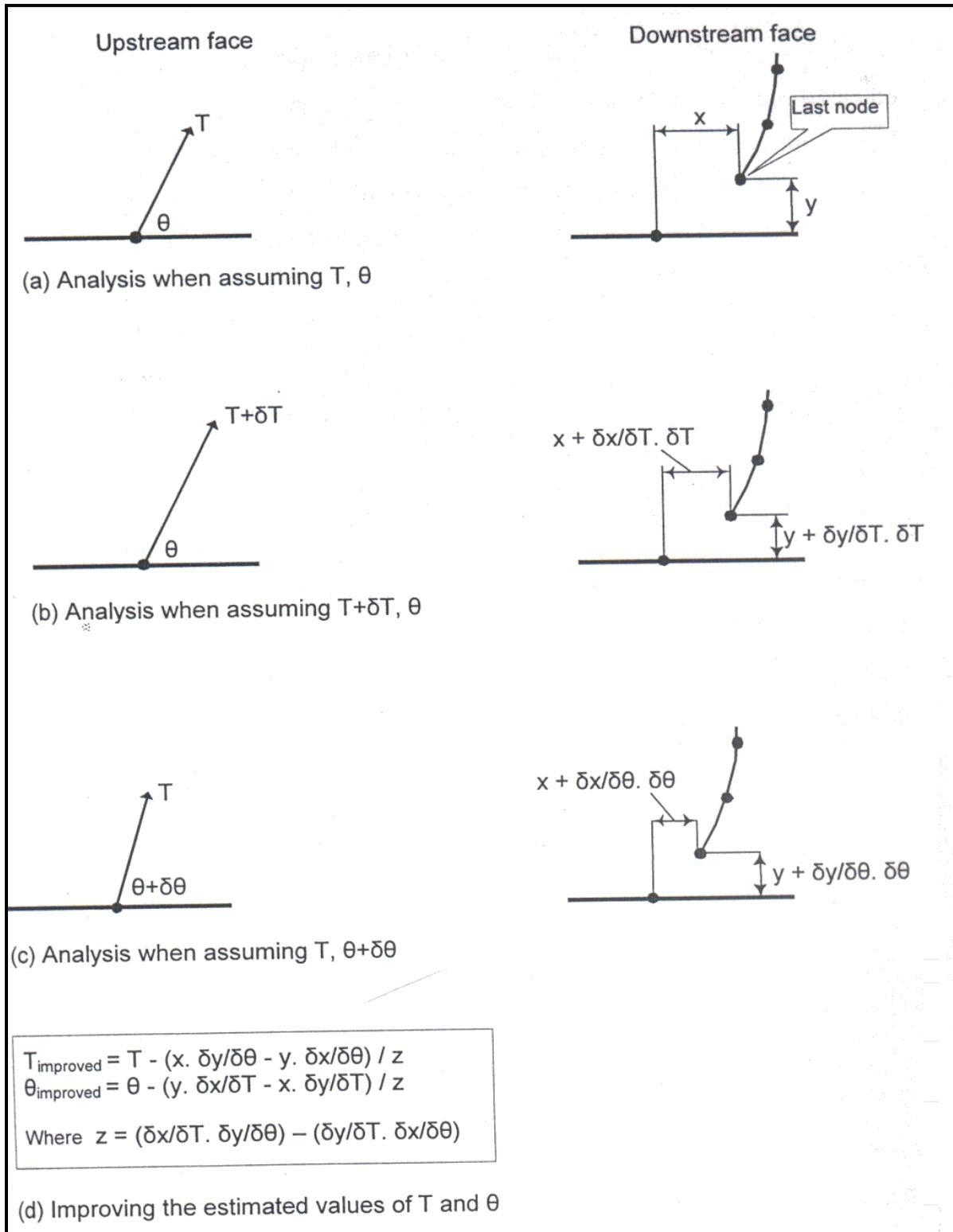
**Figure (A-3) Improving Initial T and  $\theta$  to Reduce the Miscloses**
