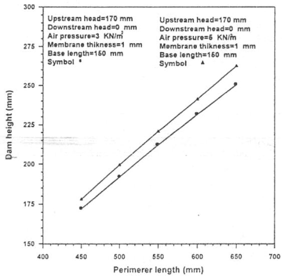
Fig.21 Variation of Dam Height with Membrane Perimeter Length (Air-inflated Dam)
