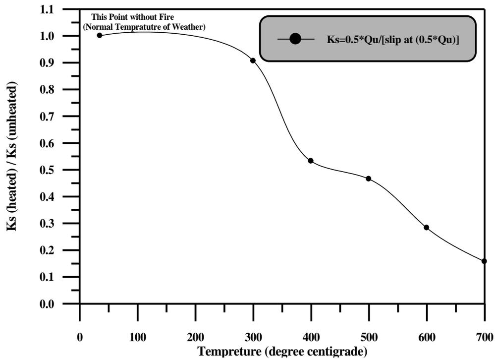
Figure (7) Connector Stiffness Ratio after Heating to Different Temperatures
