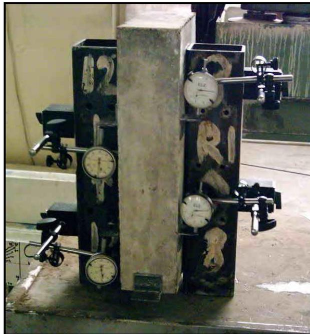
**Figure (4) Modified Push-Out Test**
