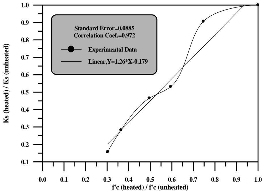
**Figure (8) Variation of Connector Stiffness Ratio with the Concrete Compressive Strength Ratio**
