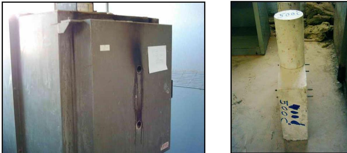
**Figure (2) Pictures; (A): An Oven of High Heating (Up to 1200 °C); (B): A Specimen to be Heated**
