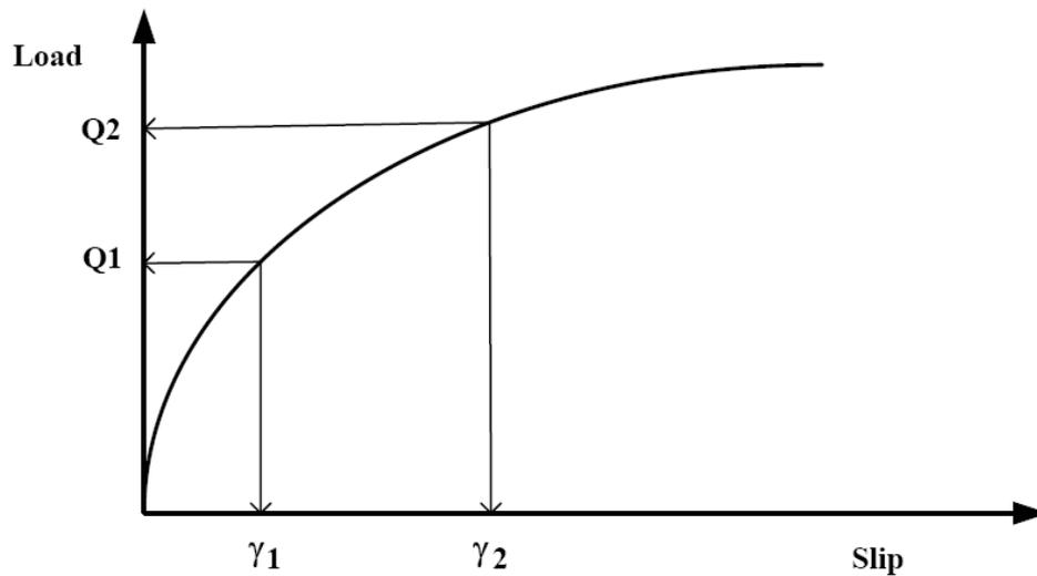
**Figure (1) Typical Load-Slip Relationship from the Standard Push-Out Test**
