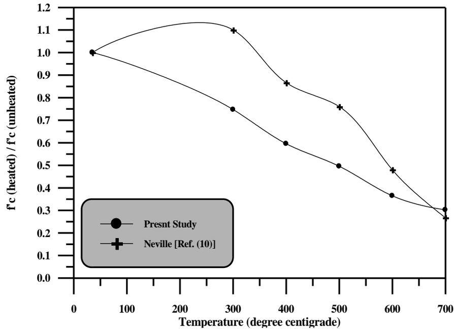
Figure (3) Compressive Strength of Concrete after Heating to High Temperatures [10]
