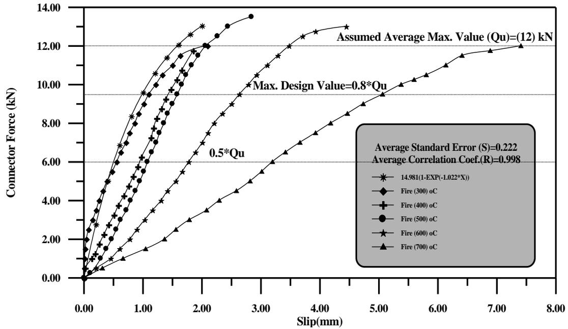
Figure (6) Load-Slip Relationship of Connector after Heating to Different Temperatures
