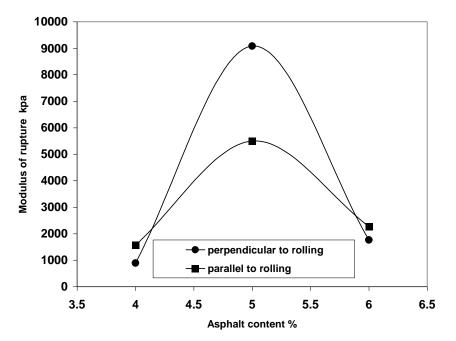
Figure (2) Modulus of Rupture of Dense Graded Asphalt Concrete
