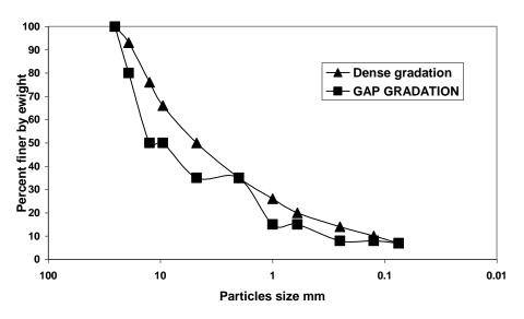
Figure (1) Grain Size Distribution of the Design Mixes
