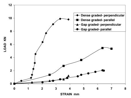
Figure (8) Typical Load-Strain Relationship at 5% Asphalt Concrete
