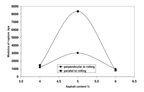
Figure (3) Modulus of Rupture of Gap Graded Asphalt Concrete
