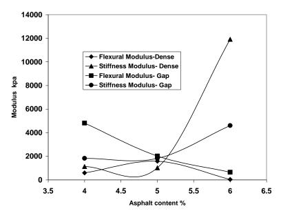
Figure (5) Modulus of Asphalt Concrete
