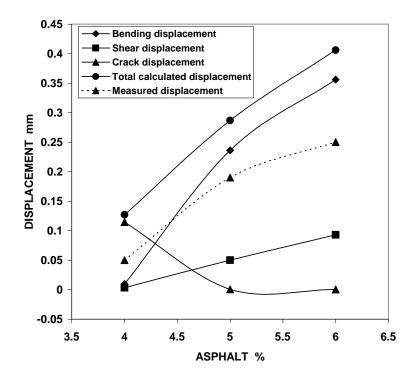
Figure (6) Displacement of Dense Graded Asphalt Concrete
