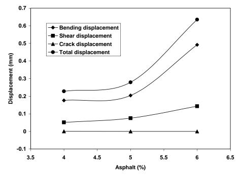
Figure (7) Displacement of Gap Graded Asphalt Concrete
