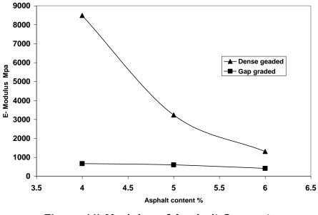
Figure (4) Modulus of Asphalt Concrete
