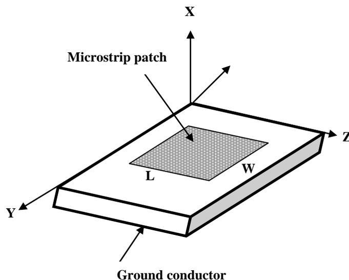
Figure (1) Microstrip antenna element
