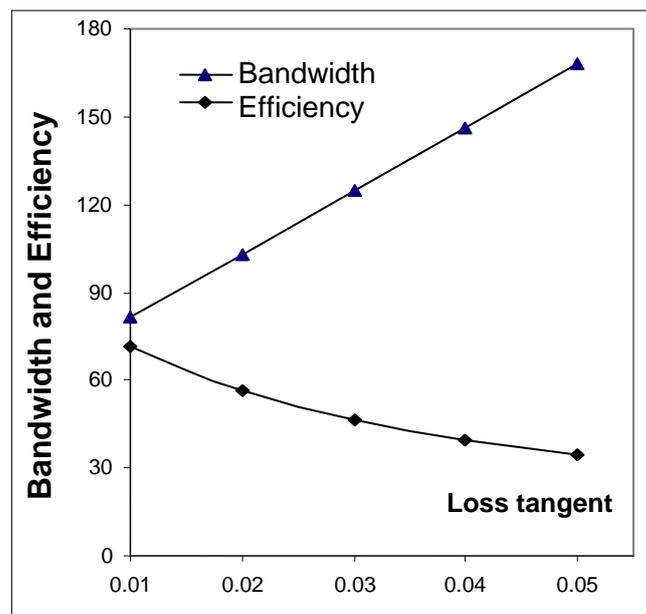
**Figure (7) Variations of bandwidth and efficiency of RMSA versus the loss tangent**
