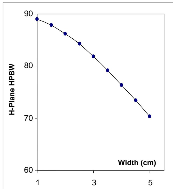
Figure (5) Variation of H-Plane half power beam width versus the patch width
