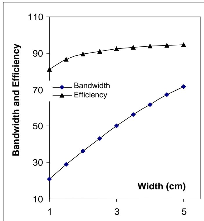
Figure (4) Variations of bandwidth and efficiency versus the patch width
