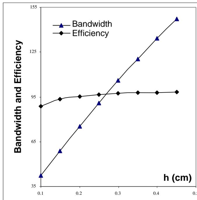
Figure (6) Variations of bandwidth and efficiency versus the substrate thicknesses
