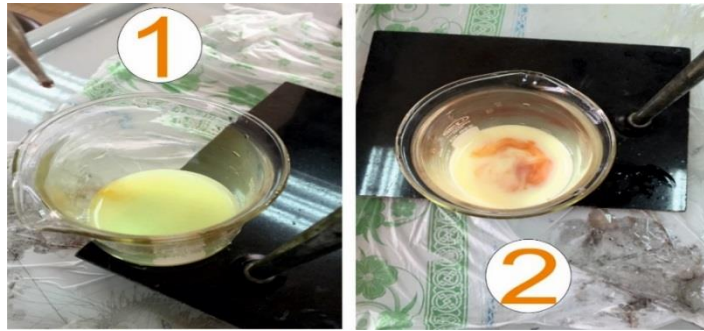
Figure (3) Titration results 1. White precipitation ( \text{AgCl} ), 2. Red precipitation ( \text{Ag}_2\text{CrO}_4 ).
