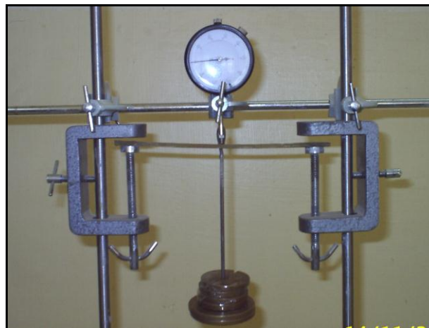
Figure (1) Flexural apparatus with specimen test
