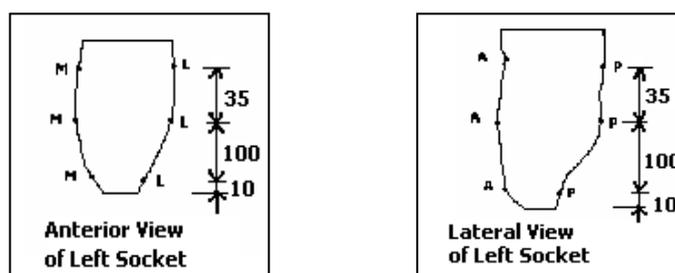
**Figure (10) Locations of evaluated stresses on the sockets**
