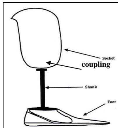
**Figure (1) The prosthesis components <sup>[1]</sup>**
