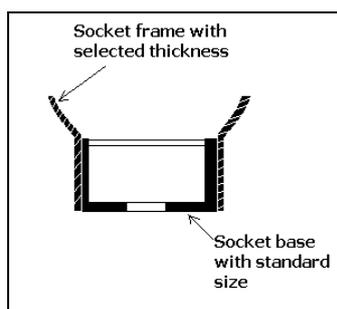
**Figure (9) Polypropylene socket base**
