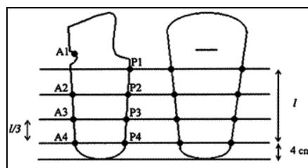
**Figure (4) Pressure transducer locations**
