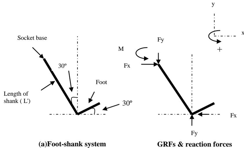
Figure (6) The foot-shank system at heel-strike [8]
