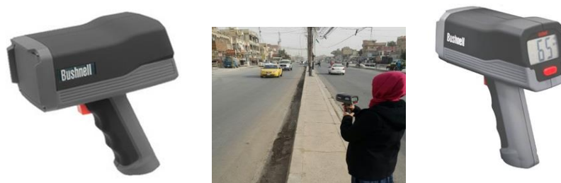
Figure 2: The speed gun using in measuring the vehicles speed
