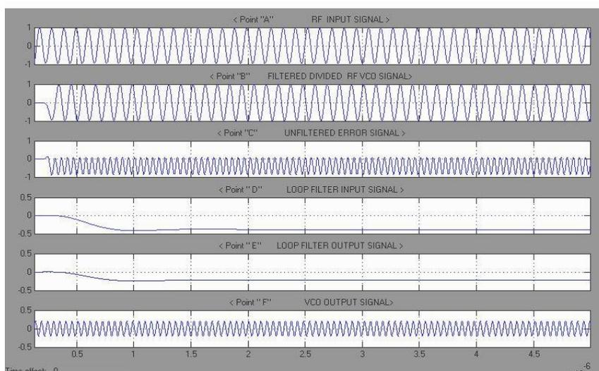
Figure (9b) Time waveforms for single main loop PLL without Doppler shift
