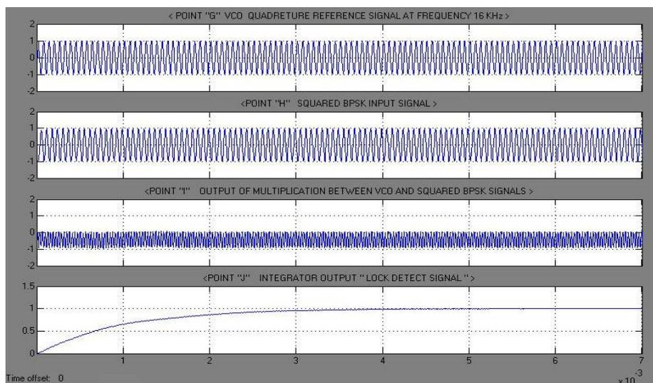
Figure (13e) Waveforms of lock indication procedure
