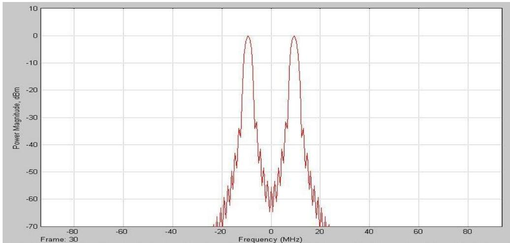
**Figure (16a) Spectrum of RF input signal at frequency of 9.375MHz**
