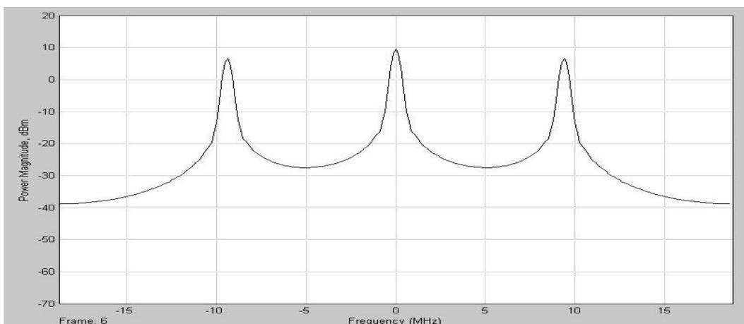
**Figure (16c) Spectrum of RF divided DVCO signal at frequency of 9.375MHz**
