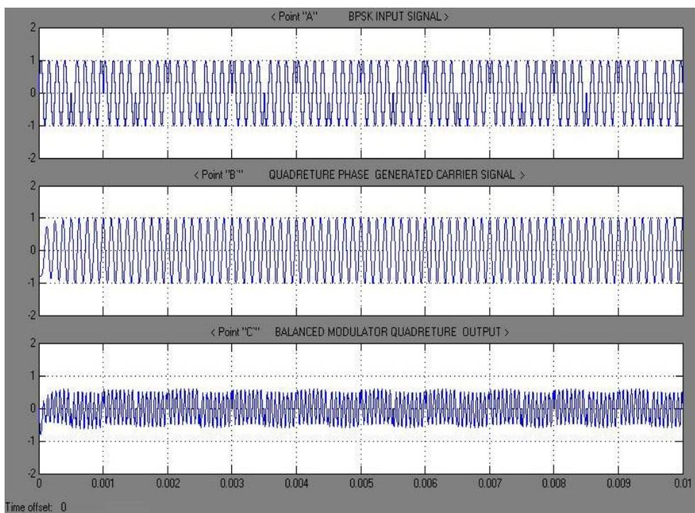
**Figure (13b) BPSK input, quadrature phase local carrier and multiplier2 waveforms**
