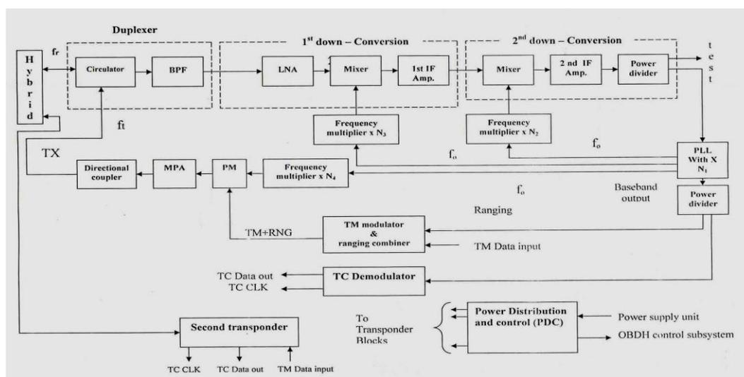
Figure (5) TMTC Transponder functional block diagram
