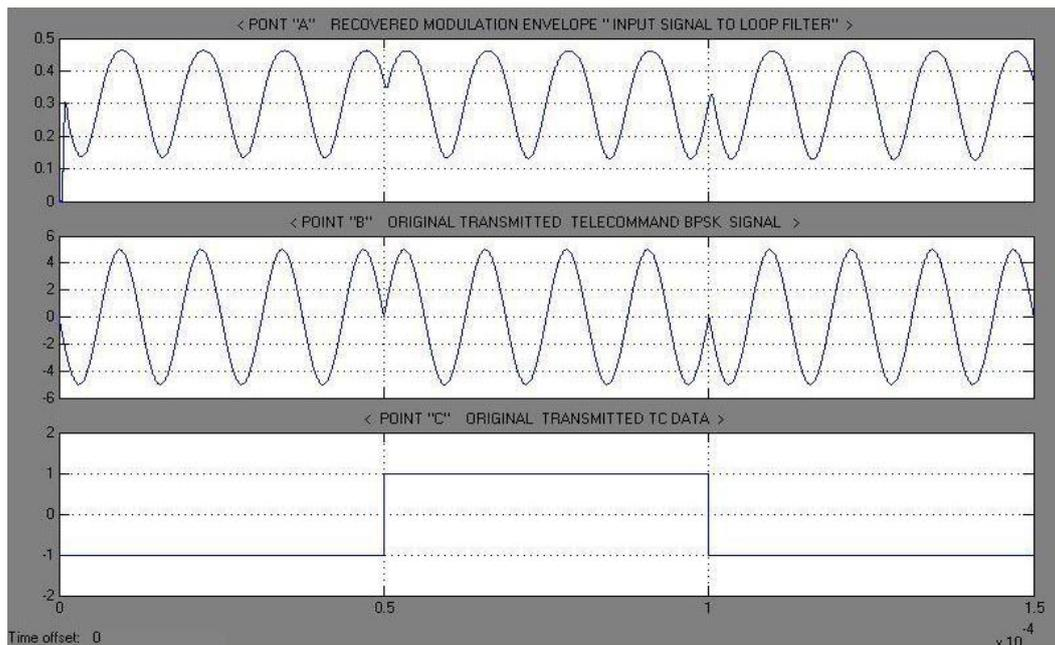
**Figure (17b) Phase detector output when BPSK phase modulated RF carrier compared with TC data**
