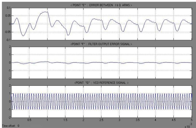
Figure (13c) Error between I&Q arms and VCO reference waveforms
