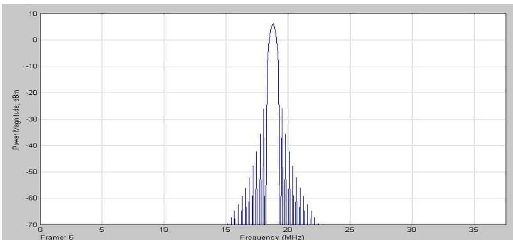
**Figure (16b) Spectrum of RF DVCO at frequency of 18.75 MHz**
