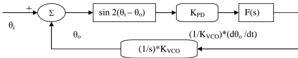
Figure (7) Equivalent PLL block diagram for a costas loop
