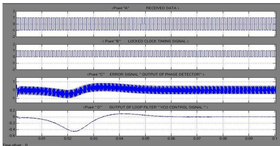
**Figure (14b) Timing waveforms for the simulated bit synchronization**
