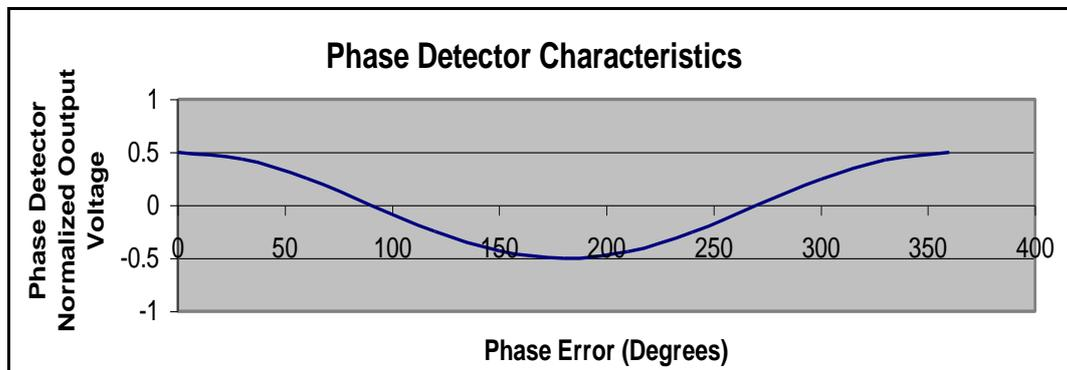
**Figure (11) Error signal amplitude versus the phase difference**
