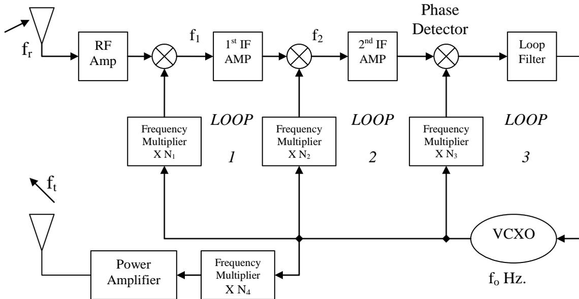
**Figure (4) Phase locked transponder**
