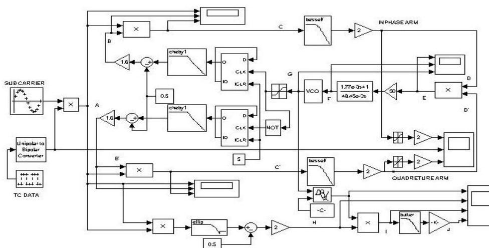
**Figure (12) Circuit diagram for Costas recovery loop and subcarrier lock indication**
