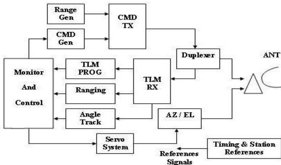
Figure (3-a) Simplified block diagram of TTC ground station
