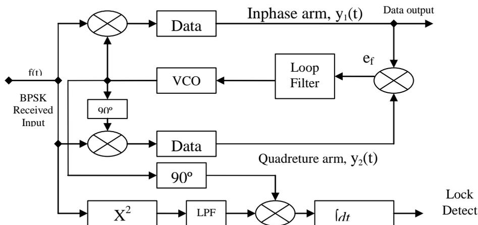
Figure (6) Typical PSK demodulation
