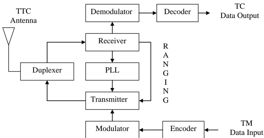
Figure (3-b) Satellite TMTTC subsystem block diagram
