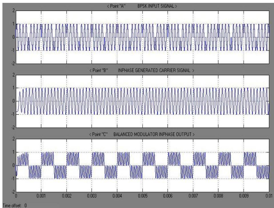
**Figure (13a) BPSK input, in phase local carrier and multiplier1 waveforms**
