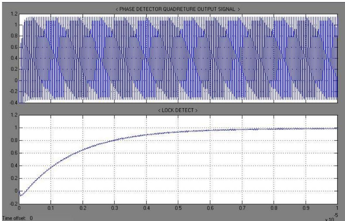
Figure (16d) Lock indication waveform
