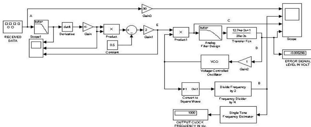
**Figure (14a) Circuit diagram for bit synchronization simulation**
