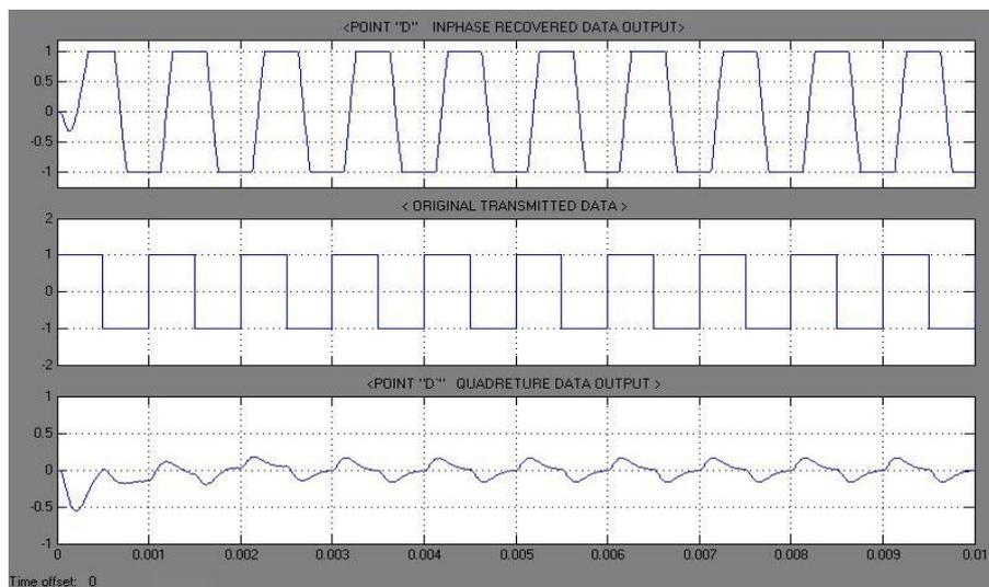
Figure (13d) I&Q arms data output and original TC data waveforms
