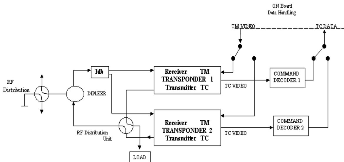
**Figure (1) Architecture of a typical spacecraft TTC system**
