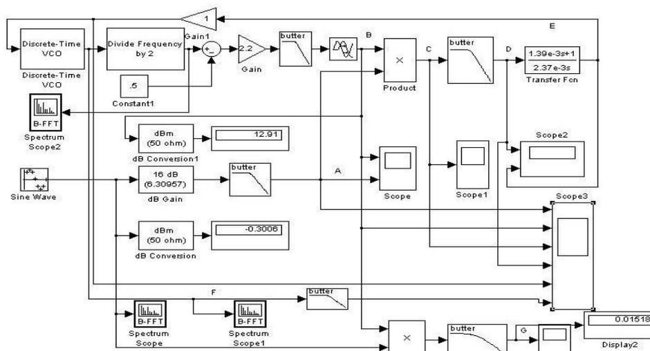
Figure (9a) Single main loop PLL circuit diagram without Doppler shift
