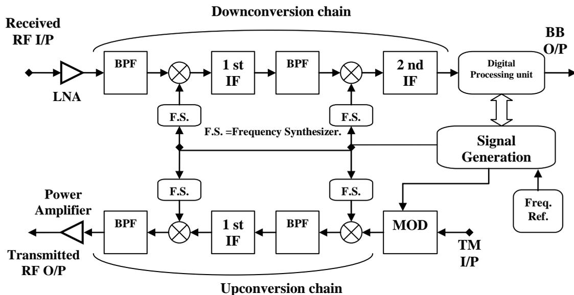
Figure (2) Block diagram of a typical TTC transponder
