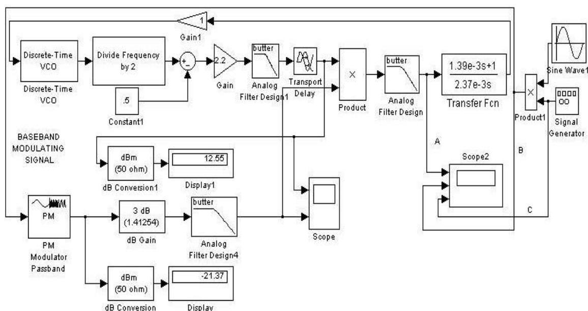
Figure (17a) Main Loop PLL unit under phase modulation
