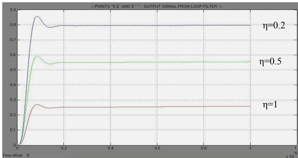
**Figure (10) Loop filter output signal versus different damping factors**
